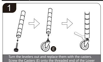
poles (D). Tighten securely with the wrench.
