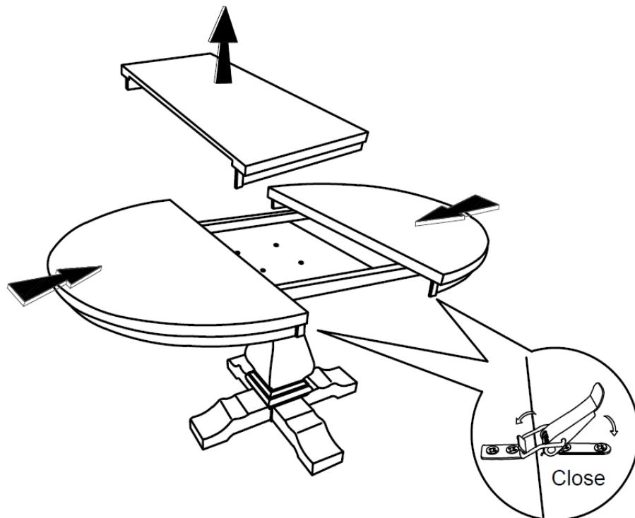
Take out the leaf. Close the Table Top (A) tightly and lock all latches underneath the Table Top (A).
