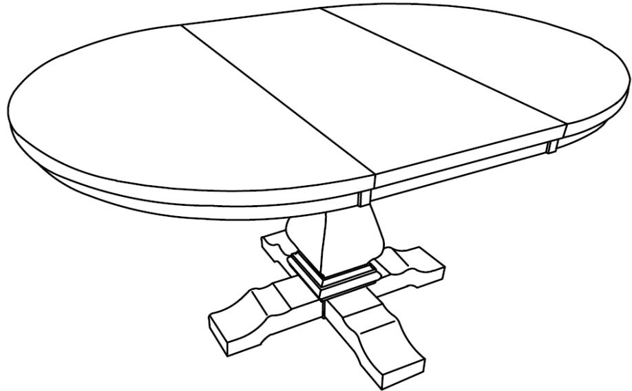
Place the Table on a LEVEL SURFACE and check that it is balanced. If there is a slight wobble, please adjust the Adjustable Gliders (9).
