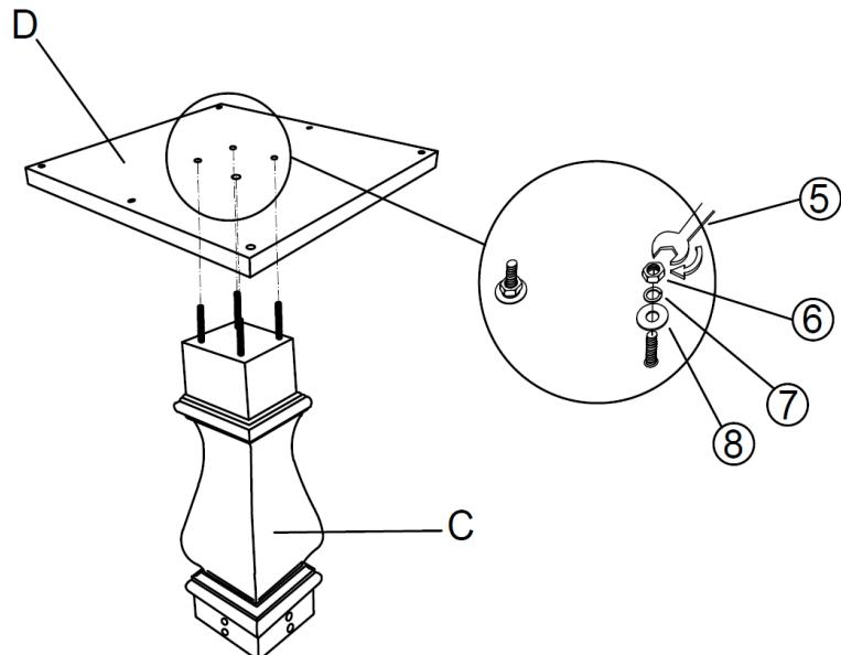
Attach the Mounting Plate (D) to the Pedestal Column (C) using Nuts (⑥), Spring Washer Rings (⑦) & Flat Washer Rings (⑧) and the Wrench (⑤).
