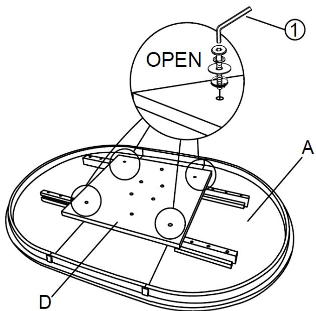
Please loosen the 4pcs Bolts, Spring Washer Rings and Flat Washer Rings from the Mounting Plate (D) using the Allen Wrench (1). Keep the hardware for Step 6.
