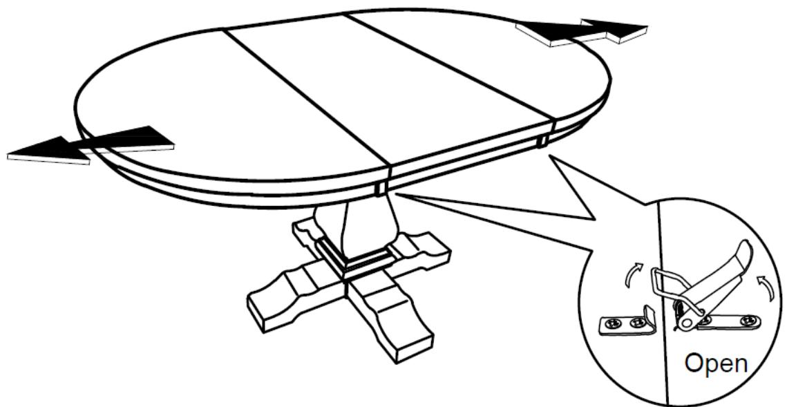
Stand the Table up with the assistance from your partner. Unlock the latches underneath the Table Top (A). Pull apart the Table Top (A) from both ends.
