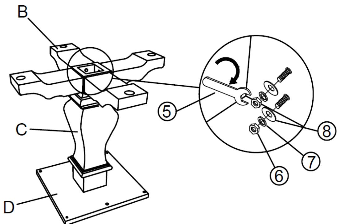
Attach the Pedestal Legs (B) to the Pedestal Column (C) using Nuts (⑥), Spring Washer Rings (⑦) & Flat Washer Rings (⑧) with the Wrench (⑤). Please assemble the Nut with the lower bolt first then the upper bolt.
