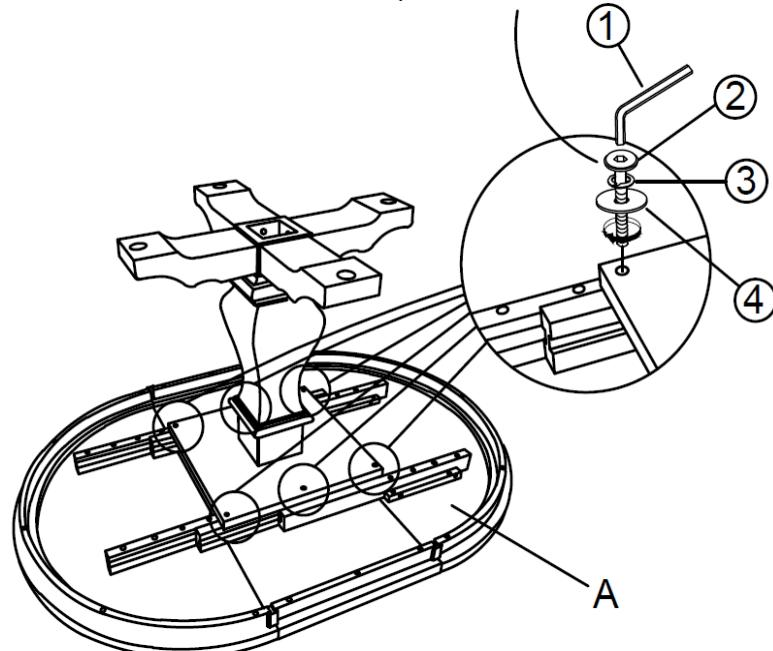
Place the the Table Top (A) on a clean non-marring surface, then place the assembled table parts from Step 5 on top of it. Affix the Table Top (A) to the Mounting Plate (D) with Bolts (2), Spring Washer Rings (3) & Flat Washer Rings (4) using the Allen Wrench (1).
