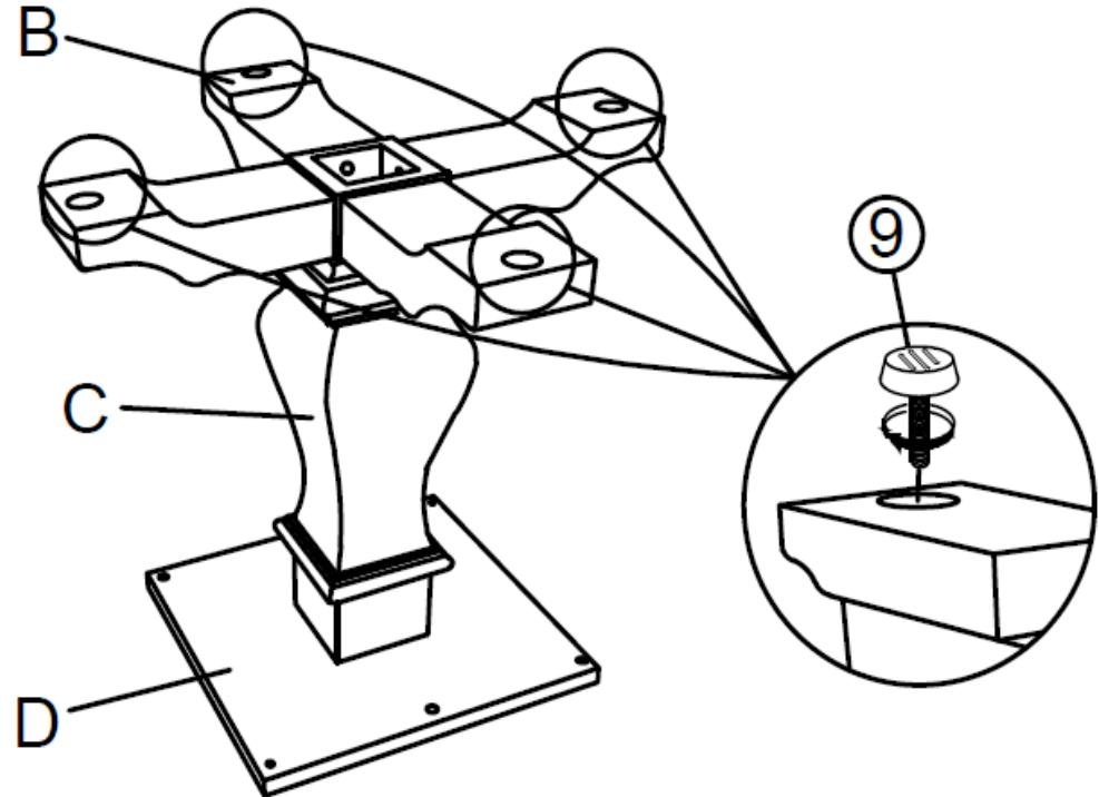
Insert the Adjustable Gliders (9) into the Pedestal Legs (B) as shown above.
