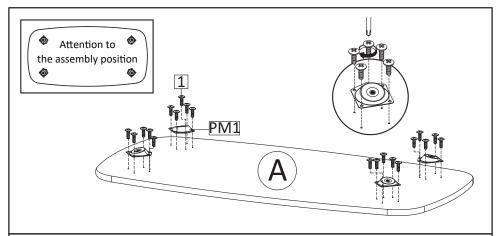
**STEP1**: Install Mounting Plate (PM1) and secure with Screw M4.5x12.5mm (HW1) on Top Board.
