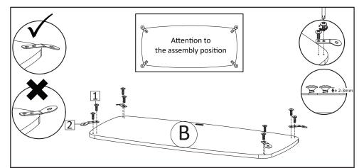
**STEP3**: Install Plate Shelf (HW2) and secure with Screw M4.5x12.5mm (HW1) on Fixed Shelf (B) position as shown in the figure. Do not overtight screw yet, leave around 2-3mm gap.
