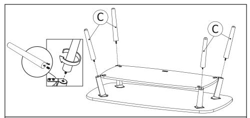
**STEP5**: Insert Leg 1 (C) into Mounting Plate, tighten by rotating, the leg clockwise. Position as shown in the figure.
