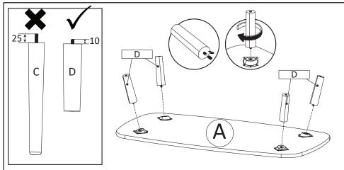
**STEP2**: Carefully see the wooden leg type needed in this step. Insert Leg 2 (D) into Mounting Plate, tighten by rotating the leg clockwise.
