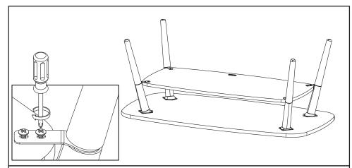
**STEP6**: Continue with tighten all screws on the Plate Shelf.
