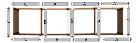
**Note:** Stacking stakes insert into the top of the previous level stakes.
