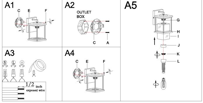
Connect wires according to the below chart
