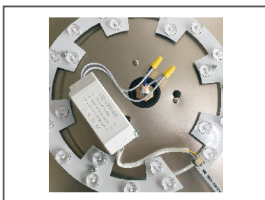
Step 3. Wiring diagram of LED light source and LED driver.
