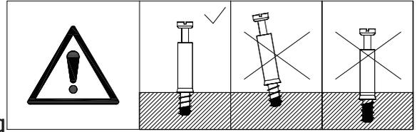
Insert quickfit screw(A) into corresponding holes in both sides of No.3 plate with a screwdriver.
