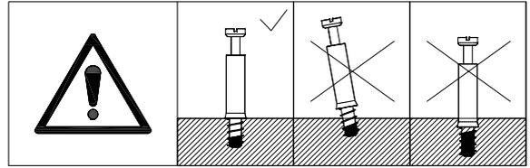
Insert quickfit screw(A) into corresponding holes in No.4 and No.2 plate with a screwdriver.
