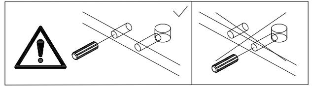
Insert wooden dowel(D) into No.2, No.3 and No.4 plate as shown.
