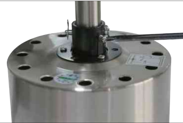
Step 8 Tighten the 2 screws on the coupler.
