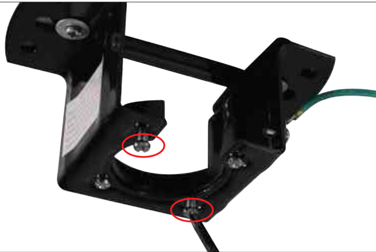
Step 10 Loosen the two opposite screws.
