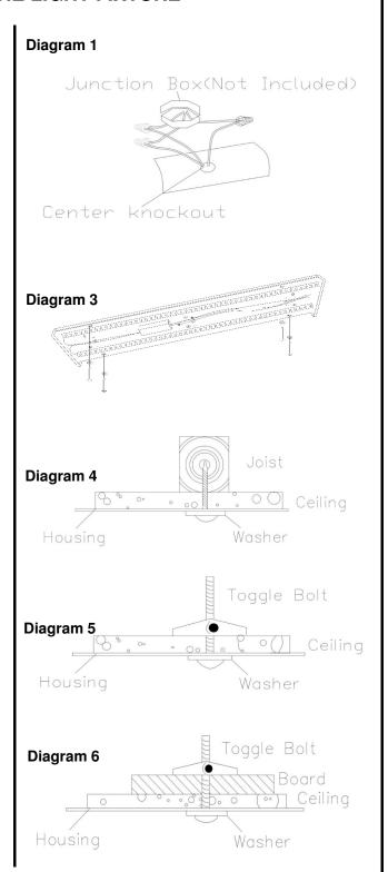
WARNING: Before wiring to the power supply, turn off the electricity at fuse or circuit breaker box. Ensure grounding to avoid potential electrical shock and to ensure reliable lamp starting.
