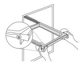
2 Keeping both levers pressed, lift the drawer support slightly and remove it from the rail system.
