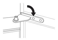
5 Tighten the two hinge bolts.
