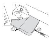
4 Position the middle hinge pin in place to hold the door and insert the two hinge bolts.
