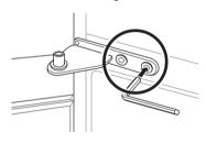
2 Twist the hinge to raise the pivoting end so that the door can be lifted off. Lift the door off the lower hinge pin and remove it.
