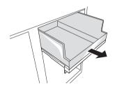
2 Lift the empty freezer drawer slightly to remove it from the support.
