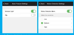
$\label{light:bound} \begin{tabular}{ll} Indicator Light: By default, the camera's light is set to remain lit to indicate power. Switch "Indicator Light" off to hide the light. \\ \end{tabular}$
