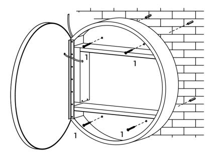
**Note:** When mounting to the wall, the wire can not be pressed between the cabinet and the wall, otherwise the wire installation will be affected.
