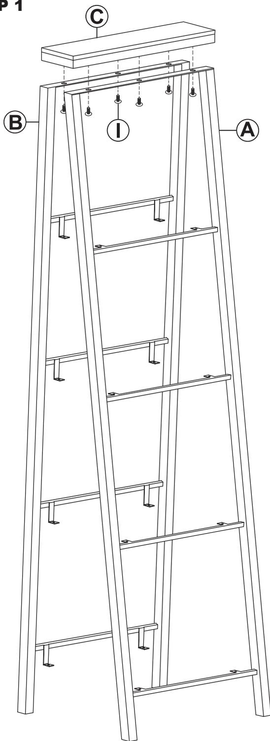
Ensuring the shelf mounting brackets face the center, align Top Panel (C) with Front Frame (A) and Back Frame (B). Loosely secure the top panel by hand-tightening six M6x10mm Bolts (I).
