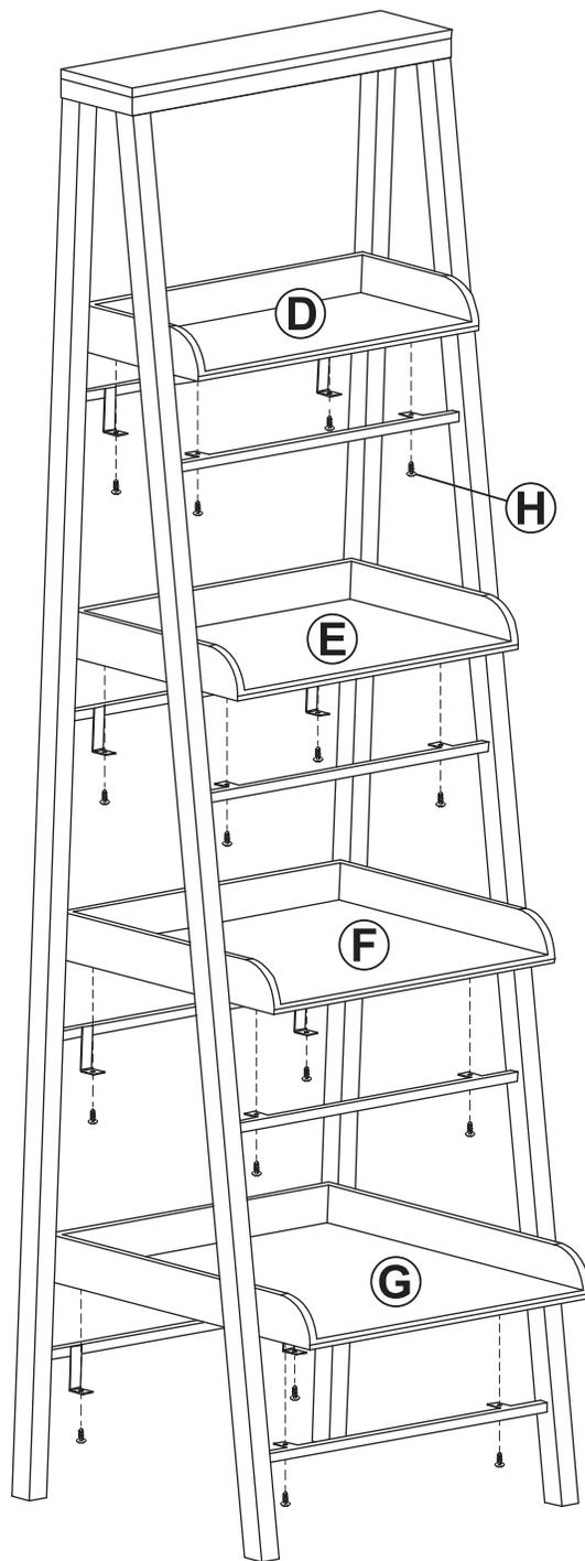
Install Top Shelf (D), Second Shelf (E), Third Shelf (F), and Bottom Shelf (G) using four M4x12mm Screws (H) for each shelf, as shown.
