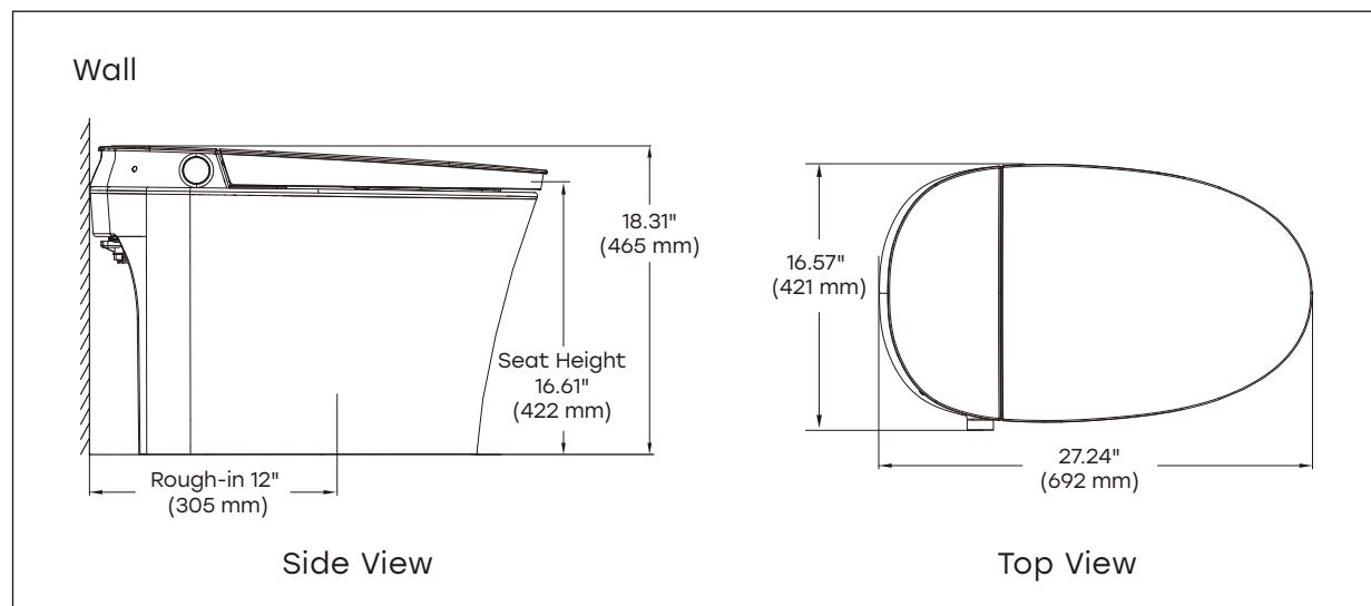
To ensure proper installation, the distance between the water supply valve and the centerline of the toilet should be greater than half the width of the toilet bottom. The water supply valve should be about 8 inches away from the toilet centerline. For larger valves, a greater distance may be necessary to ensure proper clearance. For easy installation and maintenance, a range of 9 to 11 inches is recommended.
