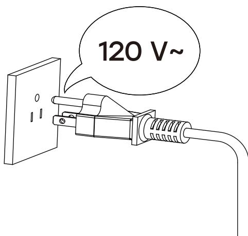
Regularly pull out the power plug and wipe off any dust on the power plug using a clean dry cloth.
