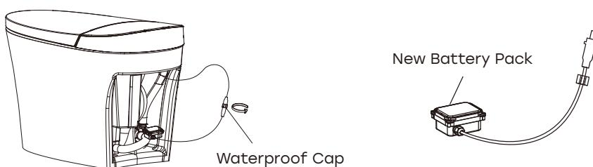
※ The battery pack for blackout flush has an IPX6 waterproof rating. A single battery pack can support approximately 200 flushes during a power outage. Please note that the battery naturally degrades over time, even when not in use.
