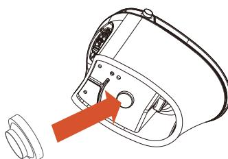
Lift the ceramic toilet with two people and gently lower it onto the flange, letting it well fit the mounting blocks.
