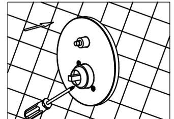
6. Lock the deck plate into the body and cling to the wall, then tight the screw.
