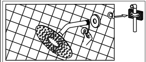
9. Install the shower arm, shower head and flange to the fitting. (stick to the wall) . Tighten the showerhead to the shower arm with the pipe tape. (Make sure the pipe tape with clockwise direction) .
