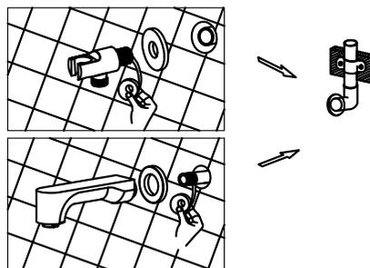
8. Wrap the thread of spout with teflon tape (ensure it must wrap clockwise). Screw-in to the inlet pipe inside the wall, then install the decorative cover on the wall clingy.
