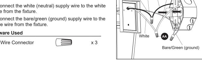
9. Wrap electrical tape (not included) around each individual wire connector (AA) down to the wire. Turn the spliced/taped wires upward and gently push the wires and wire connectors (AA) into the outlet box.
