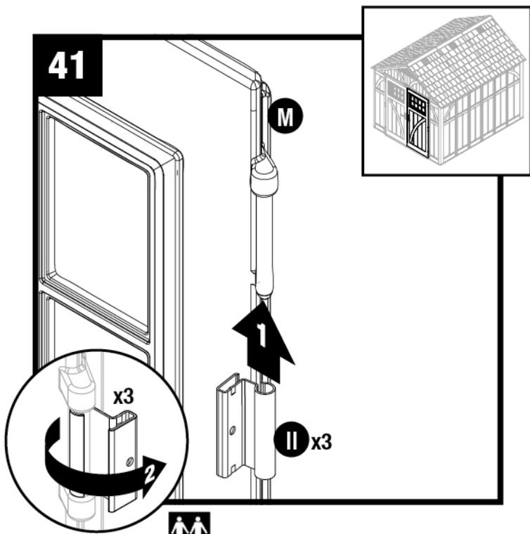
Stand right door (M) upright with three hinge mounts facing right. Slide one metal door hinge (II) up onto each hinge mount. Rotate door hinges to outside of door.
