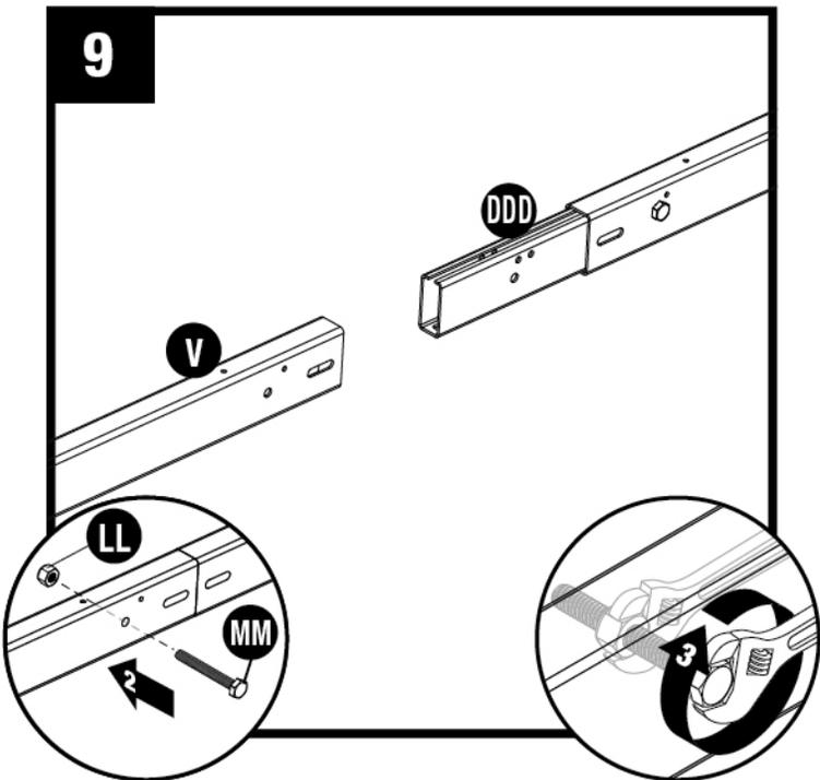
Place 7' ridge beam (V) onto the ridge beam joiner (DDD). Secure with hex bolt (MM) and nut (LL).
