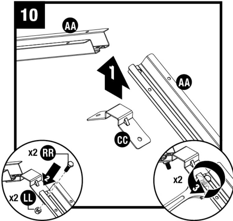
Attach truss bracket (CC) to end of one truss leg (AA) with one hex bolt (RR) and one nut (LL). Repeat for second truss leg (AA).
