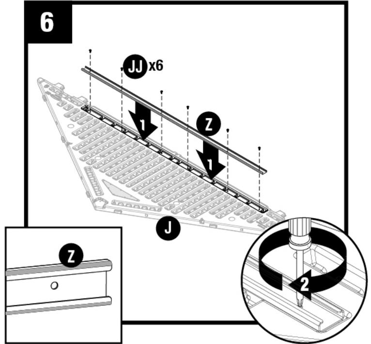
Place header beam (Z) into pocket of front header (J). Secure with six screws (JJ). **DO NOT** over tighten screws.
