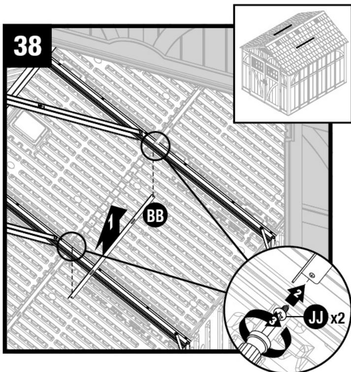
Attach roof support extension (BB) to truss legs with one screw (JJ), each side.
