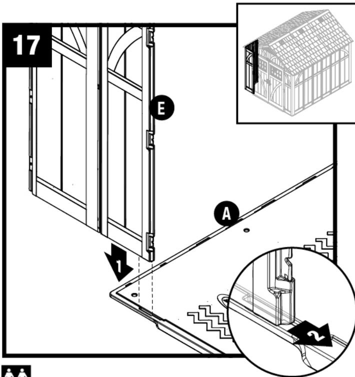
Align tab on bottom of left front corner (E) with slot on left floor (A). Lower panel into slot and lock in place by sliding panel toward door opening.
