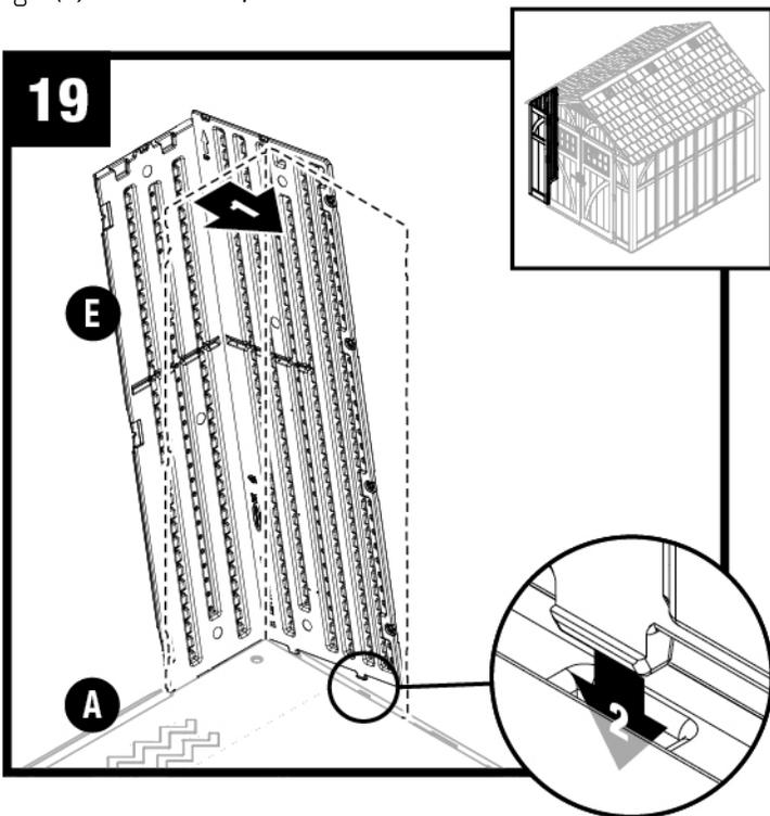
Tip left front corner (E) back to vertical position and align lower tabs on right side with slots in floor.
