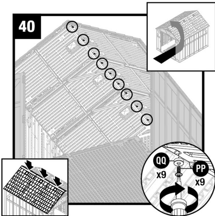
Push down the roof from outside. From inside shed, secure roof panels together along ridge of roof using nine rubber washers (QQ) and nine sealing screws (PP).
