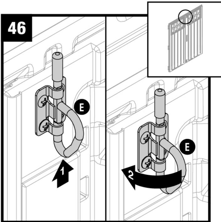
Push D-ring (E) up to engage with slot in header. Turn D-ring to left for locked position.
