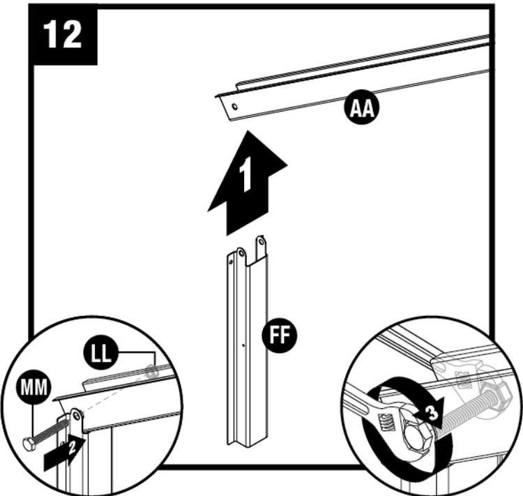
Attach side adaptor bracket (FF) at end of left truss leg (AA) with one cap screw (MM) and one nut (LL). Repeat for remaining side adaptor bracket (FF).
