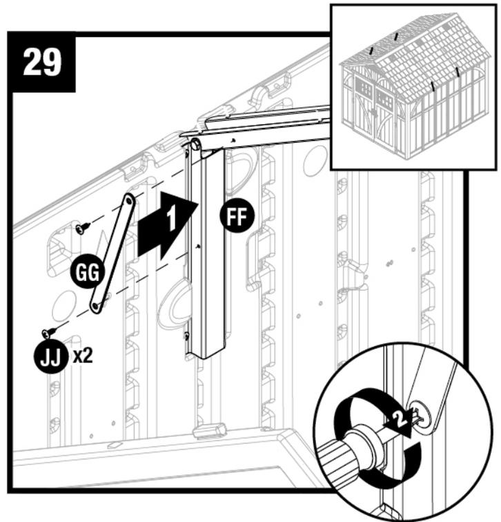
Attach truss strap (GG) to side adaptor bracket (FF) with two screws (JJ).
