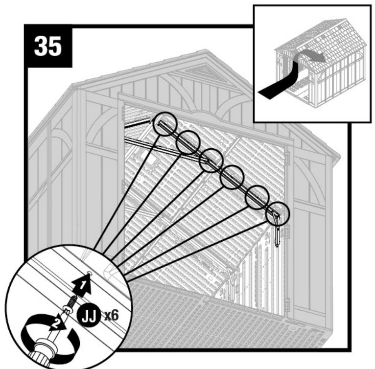
Pull down each lower corner of roof from outside. From inside shed, attach tabs on right front corner (I) and side panel (F) to roof panel with four screws (JJ).
