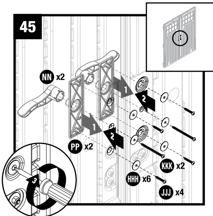
From the outside of doors, insert door handles (NN) onto the handle plates (PP). On inside of the doors, place washers (HHH) on center door handle locations, and secure each handle (NN) with one long screw (KKK).
