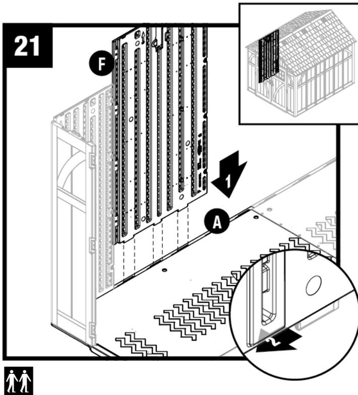
Align tabs on bottom of side panel (F) with slots along floor (A). Lower panel into slots and lock in place by sliding panel toward front corner.
