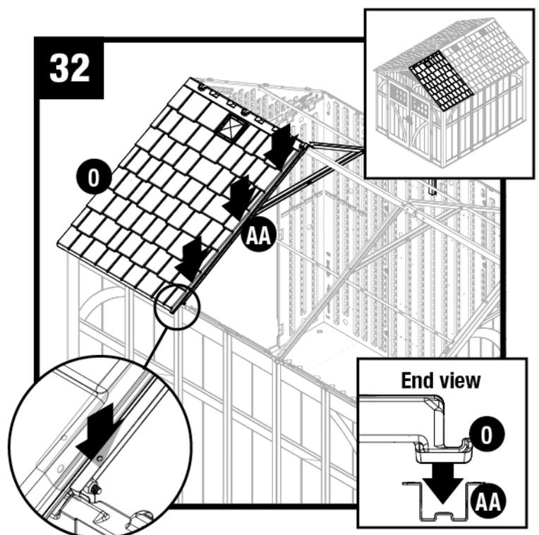
Press edge of right roof (O) into channel on truss leg (AA).
