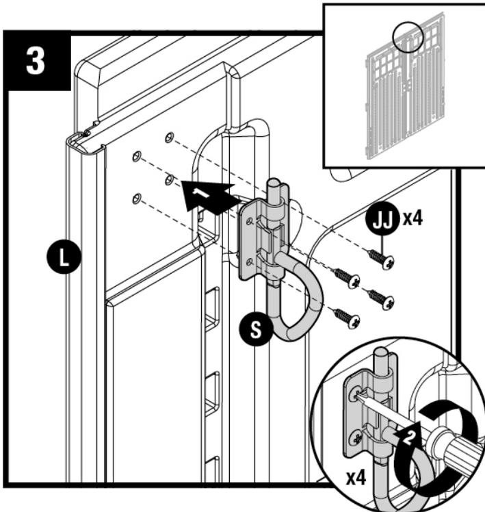
At top interior side of left door (L), attach D-ring slide bolt (S) with four screws (JJ).
