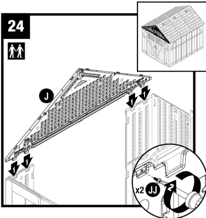
Place front header (J) over door opening and fit four protruding support legs into pockets molded in front corners. Secure front header using two screws (JJ).
