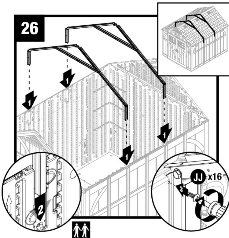
Slide truss assemblies into place. Secure with four screws (JJ) in each side adaptor bracket.
