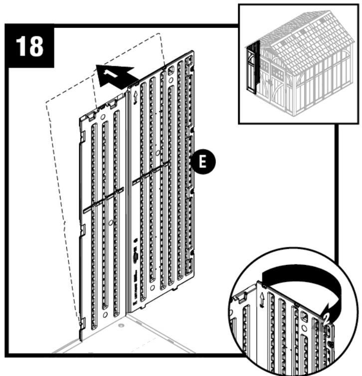
Tip left front corner (E) outward slightly and bend corner hinge.
