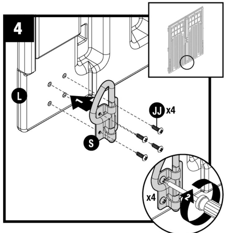
At bottom interior side of left door (L), attach D-ring slide bolt (S) with four screws (JJ).
