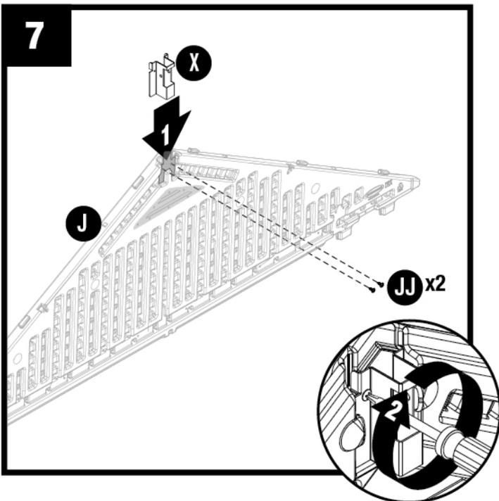
Slide roof ridge beam bracket (X) under tabs on inside peak of front header (J) and secure with two screws (JJ). **DO NOT** over tighten screws.
