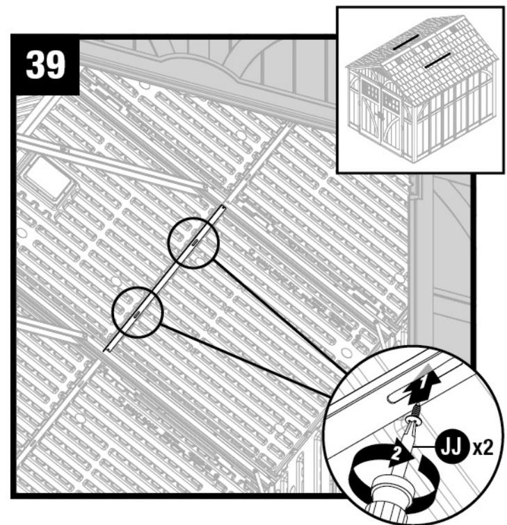
Secure roof support extension (BB) to inner roof panel using two screws (JJ).
