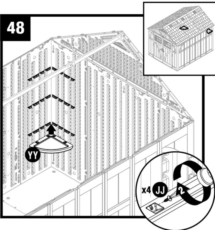
Attach shelf (YY) in desired location with four screws (JJ)
