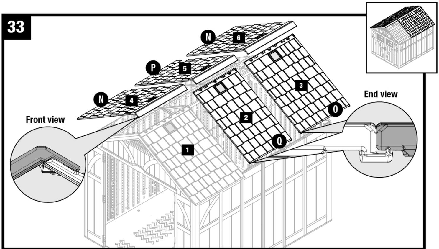
Repeat Steps 30-32 for remaining roof panels. Install panels in the order shown. **Note: At this point, fully tighten ALL hardware.**
