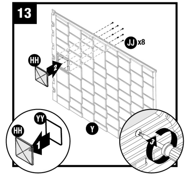
Place skylight gasket (YY) into skylight (HH). Place skylight (HH) onto right roof panel (O). Secure from underside with eight screws (JJ). Make sure rib on plastic parts is seated fully against gasket on skylight. Repeat for remaining roof panels.
