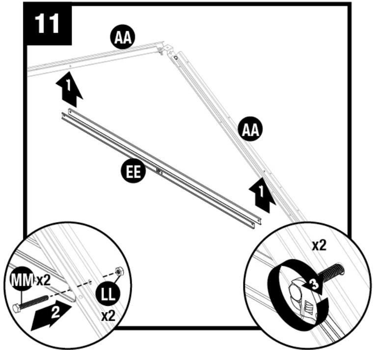
Attach two truss cross beams (EE) to two truss legs (AA) with two cap screws (MM) and two nuts (LL). Stand truss and check cross beam is level.
