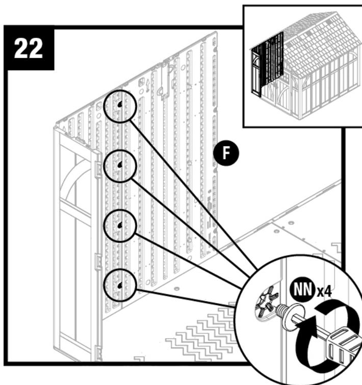
Secure side panel (F) with four easy bolts (NN), working from floor to roof. **DO NOT** use torque wrench. Use easy bolt easy driver (OO) and hand tighten. Easy bolt head will be flush when fully seated. **DO NOT** over tighten easy bolts.
