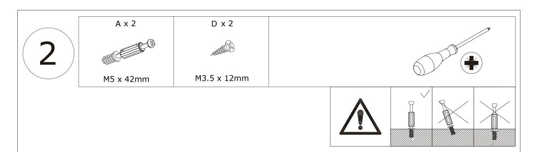
Fix No.13 slide rail to No.4 plate with screw(D) as shown. Insert quickfit screw(A) into corresponding holes in No.4 plate with a screwdriver as shown.
