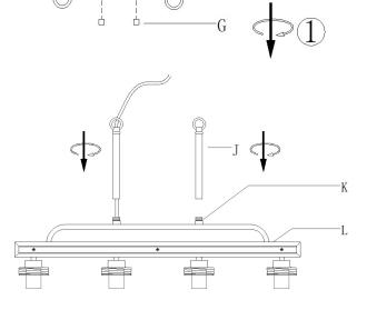
Slip the tube (L) along wires then thread onto the nipple of the top fixture body (M)till snug ,thread another tube(L) onto the nipple of top fixture body (M)till tight.
