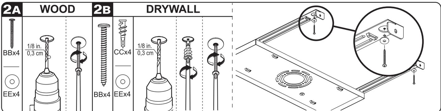
**2A** Locate the open holes for mounting at the corners of the mounting plate and drill 1/8 in. pilot hole in the center. If a wooden stud is encountered, use the screws (BB) and washers (EE) provided to secure the mounting plate directly to stud.
