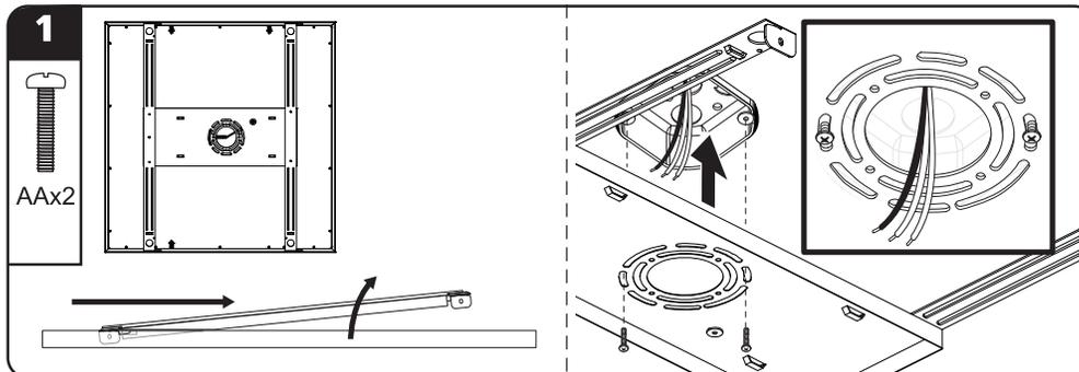
**1** Remove mounting plate from LED panel by sliding into the direction of the slots closest to the mounting screws (AA), and then lifting up. Hold the mounting plate up to the junction box in the desired fixture mounting orientation. Pull black, white and ground supply wires from electrical box through the hole in center of mounting plate. Ground wires can be either green or bare copper. Attach mounting plate to the electrical box using mounting screws (AA) provided.
