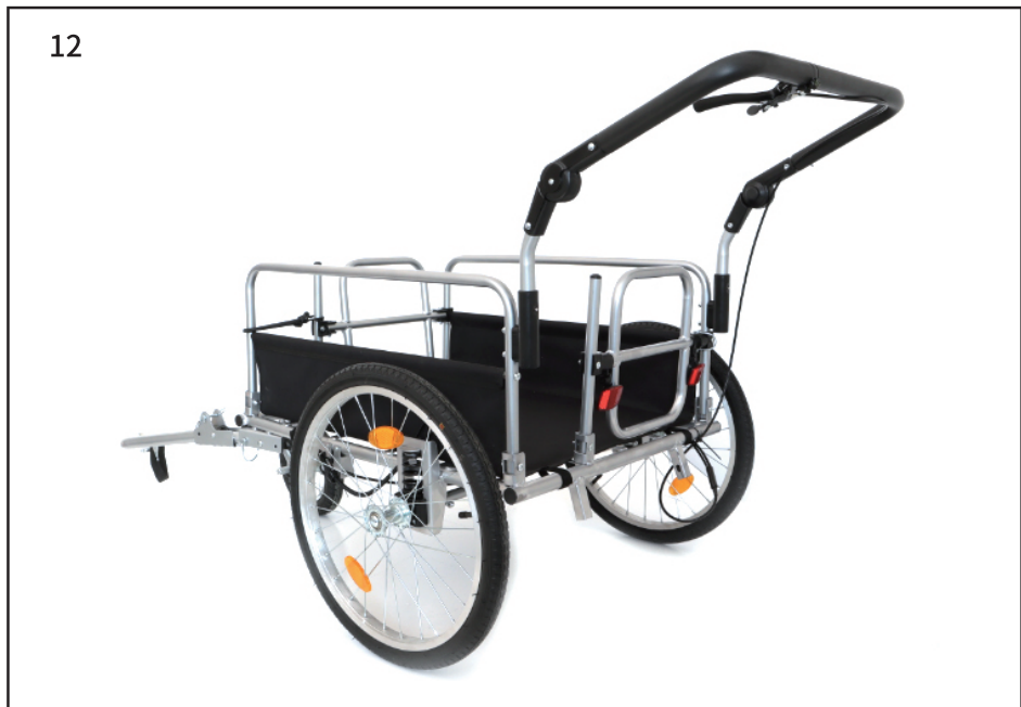
Unfasten D ring on pull handle, pull the handle out then fix with D ring when you use as trailer
