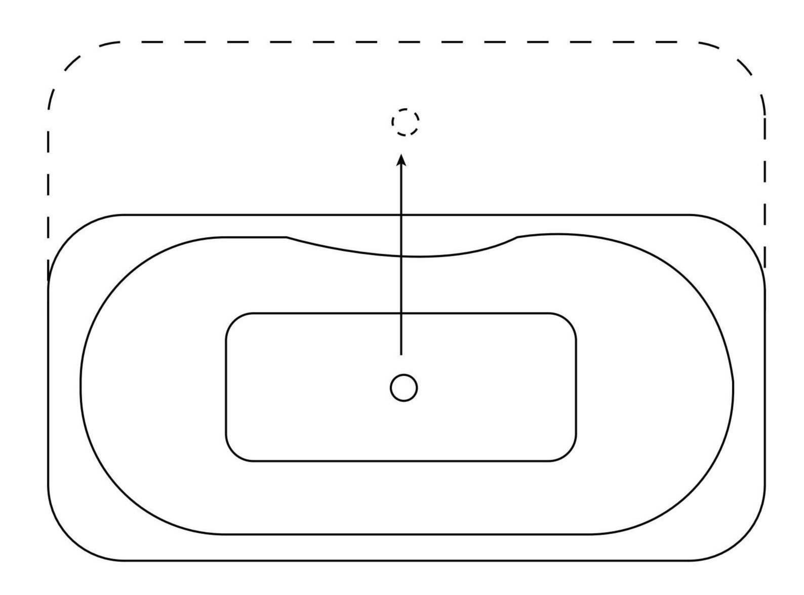
3. Place a level across the bottom of the tub to represent floor level. Raise adjustable leveling supports to touch level. Then, raise the support an additional 1/8" to ensure the bathtub is supported by the support feet and not by the tub walls.
