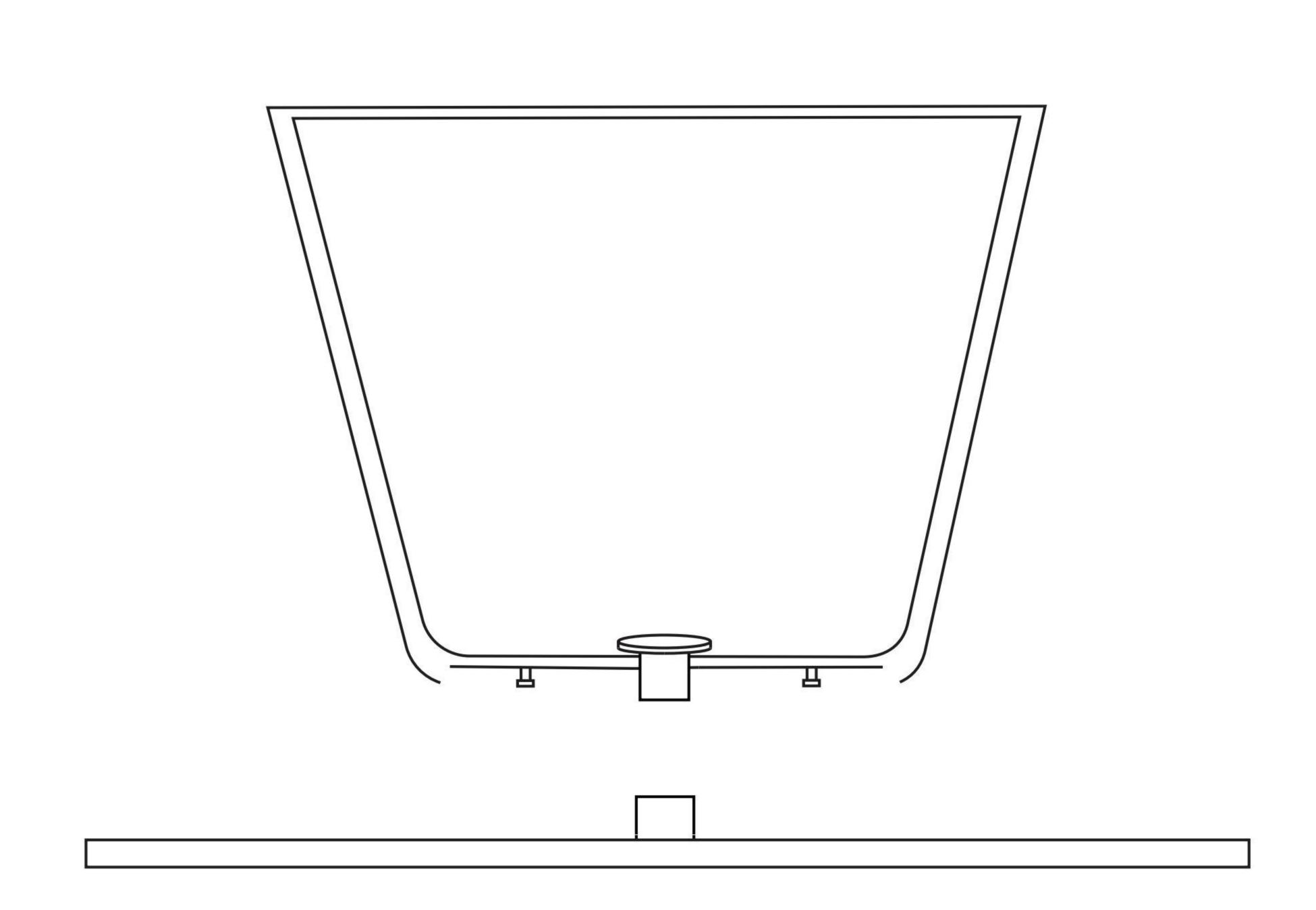
10. Fill the tub with water to check for any leaks from the connections. Verify that the drain is working properly
