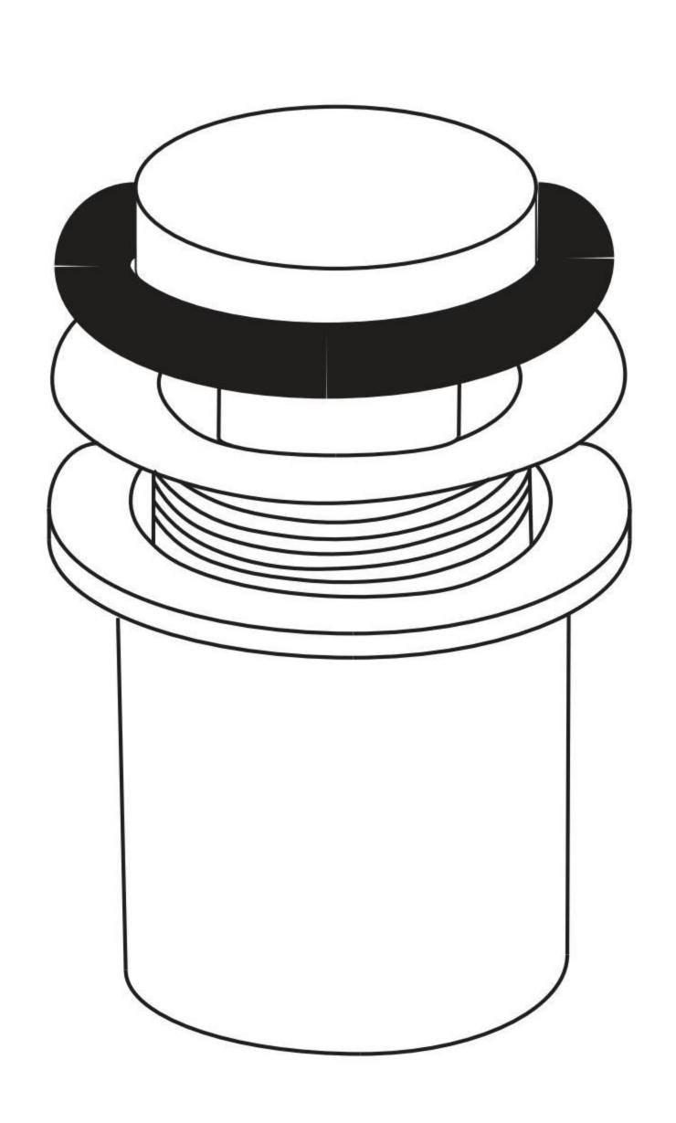
6. Your tub may come with a drain cover and pop up mechanism already installed. If not, to install the drain pop up mechanism and drain cover, simply screw the pop up mechanism into drain cap. Then, install the assembly into drain basket.
