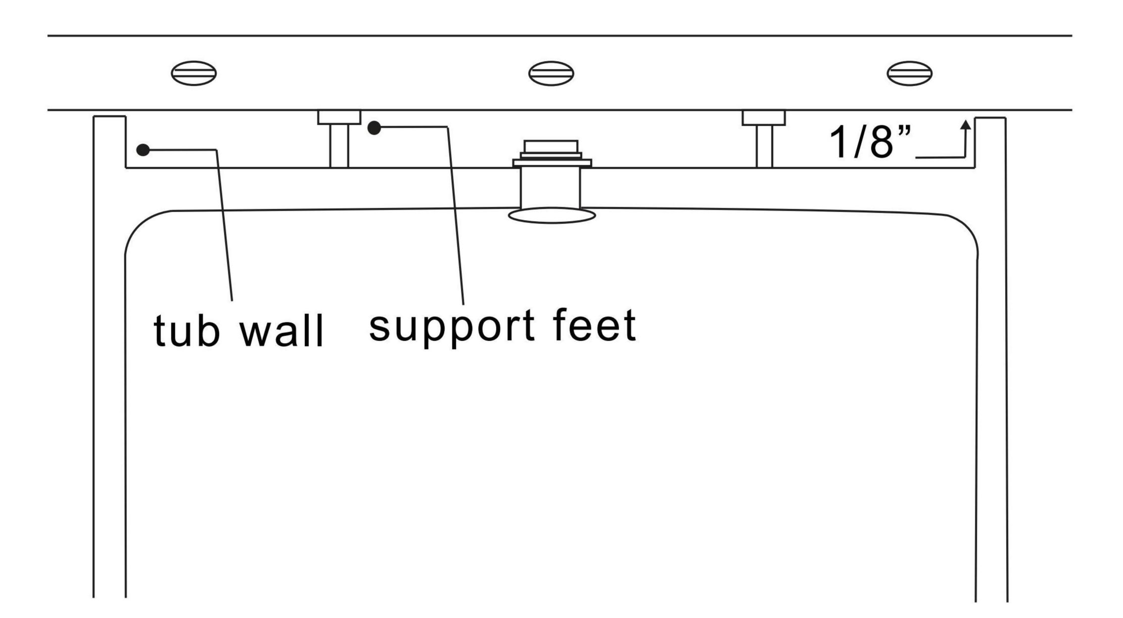
2. Turn bathtub upside down and rest it on a moving blanket, cardboard, or other soft surface to prevent scratching the rim. Use caution when turning the bathtub upside down, as the product may be heavy and may require assistance to rotate.
