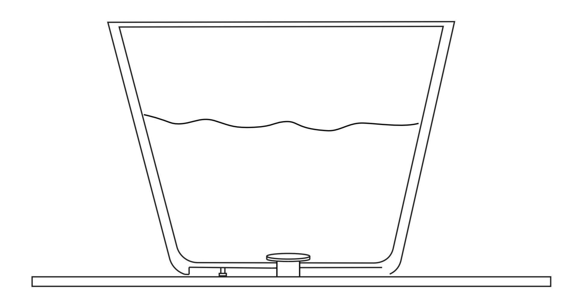
11. Finish your installation by running a bead of neutral cure silicone sealant around the base of the tub where it meets the floor. Wipe away any excess sealant with a damp cloth.
