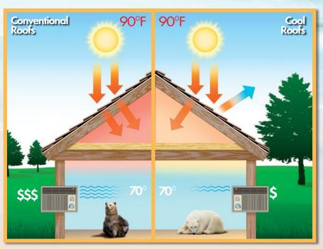
A cool roof from GAF helps minimize solar heat gain by reflecting incoming sun rays and re-emitting the absorbed energy — thereby reducing the heat going into the house and in the attic. This may translate into savings on air-conditioning bills.
