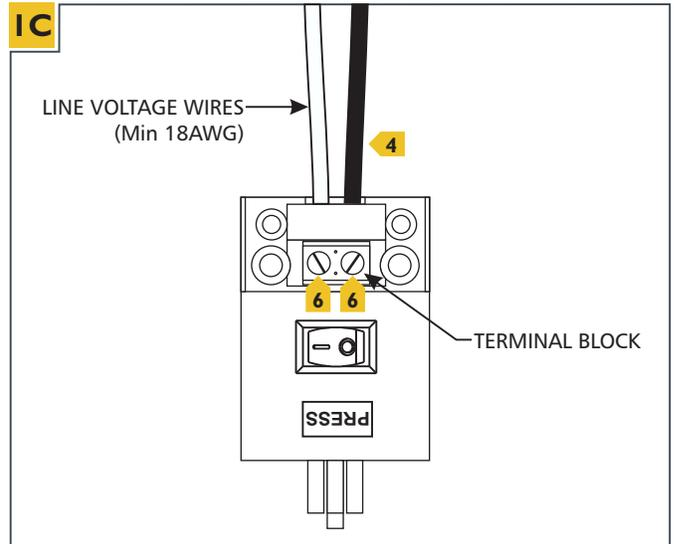
**Note:** This transformer does not require connection to a supply ground wire to insure safe operation. It is manufactured using a polymeric enclosure that provides complete isolation. If using three conductor supply wires, please sever the ground conductor cleanly so it terminates in the transformer wiring compartment.
