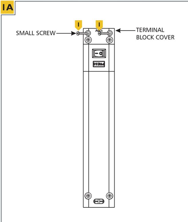
**I** Loosen (do not remove) the two small screws on the terminal block cover. Remove the cover.
