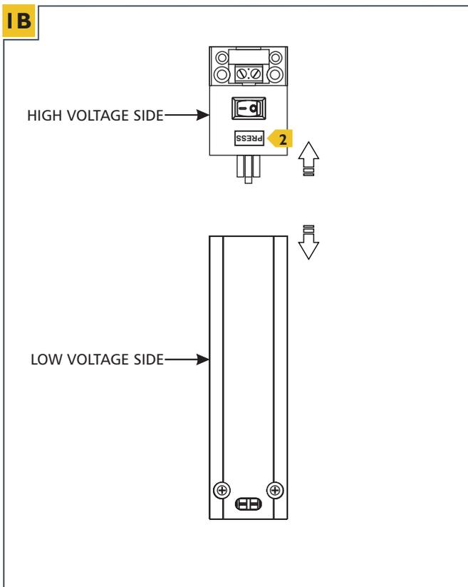
**2** Press and hold the "Press" button on the line voltage side and pull it apart from the low voltage side.
