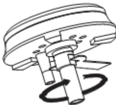
Tighten the pipe with wrench
