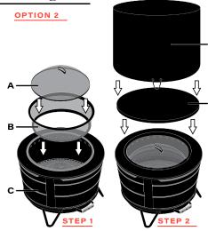
If you have purchased the tabletop as well, you may nest the screen pieces (A) & (B) inside of the Fire Pit (C), then place the stainless tabletop (E) on top. Finally, place the cover (D) (included with the Fire Pit purchase), over the top.
