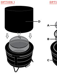
When the Fire Pit is not in use, place the cover (D) (included with the Fire Pit purchase), over to help protect your screen and Fire Pit from the elements.
