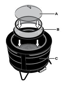
Place both top (A) and bottom (B) pieces of the screen on the Fire Pit (C). Ensure that they are securely nested.
