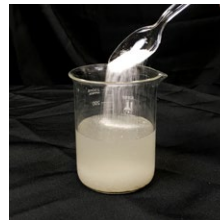
Add Liquid Lock to slurry liquid
