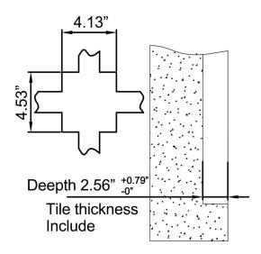
3). Put the product body into the pre-embed slots and be close to the bottomplane of the groove. Check the level meter that comes with the product, and adjust the bottom of the groove so that the air ball in the level can be in the horizontal line.
