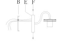
Attach the mounting plate assembly(B) to outlet box with mounting screws (D).
