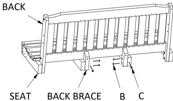
**2)** Attach Back Brace to Seat using (2) B bolts on each Back Brace.
