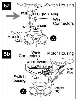
6. Wrap electrical tape (not included) around each individual wire connector down to the wire.
