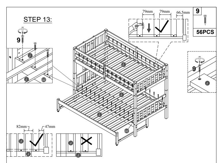
Note: Do not lock the screws of the bed slats to the outermost edge of the bed slats, you need to leave a certain space at the edges, otherwise it will cause the board to break.
