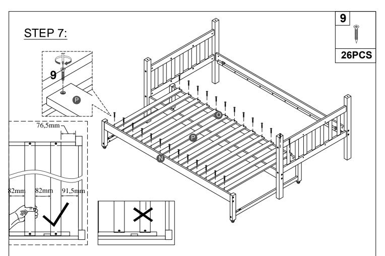
Note: Do not lock the screws of the bed slats to the outermost edge of the bed slats, you need to leave a certain space at the edges, otherwise it will cause the board to break.
