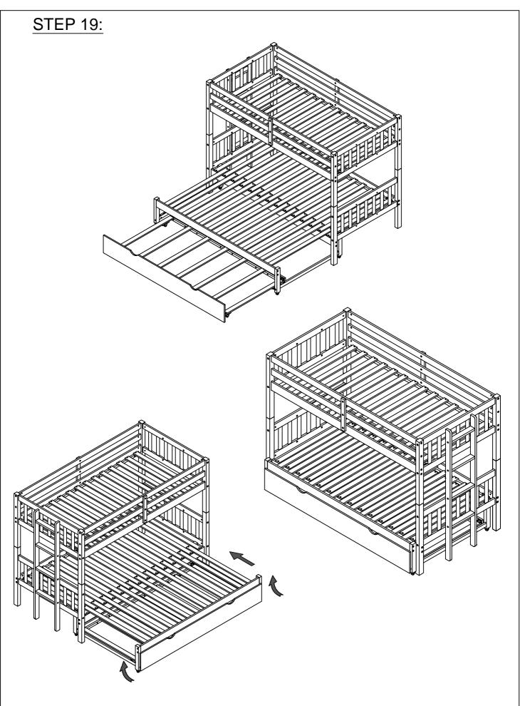
Remark: When opening or closing the pull bed, Please lift the pull bed slightly before opening or closing it.
