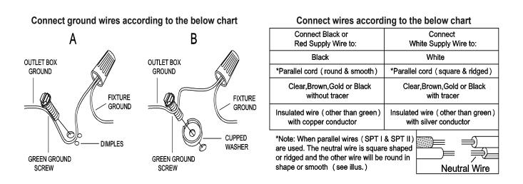
Twist wires together with plastic wire connectors until tightly joined, and wrap each connector with approved electrical tape. Be sure that no wire strands are exposed and then carefully tuck all wires into the outlet box.
