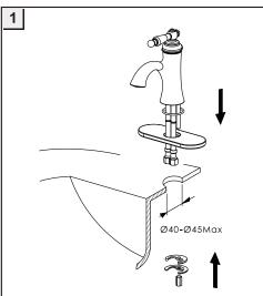
1. Make sure there is a Ø40-Ø45 Hole on the basin before fix the mixer, Unscrew the fitting ASSY from the bottom of the body, then get the body through the hole, don't forget to fix the o-ring between the bottom of the body and the basin.
