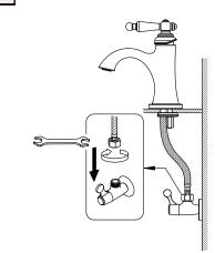
3.Connect the inlet hose from the body,"Red" for connecting to the hot water, and "Blue" for connecting to the cold water.
