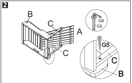
Step 2: attach the support (C) to the Seat (B) by using the Allen Screw S (G5) and tighten it with the Allen key (G8) as shown on the picture.
