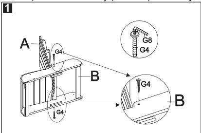
Step 1: put the back (A) inside the seat (B) use the Allen Screw L (G4) to attach it to the chair by using the Allen Key (G8) as shown on the picture.
