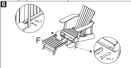
Step 5: put the foot rest (F) under the seat of chair and make sure attach the pin for lock footrest as shown on the pictures "Pic1" and " Pic 2".
