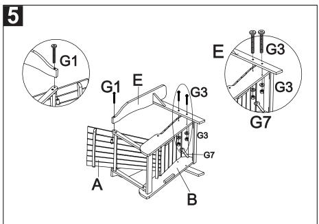
Step 4: attach the left side (D) as shown on the picture by using the Allen Bolt L (G1) and the Allen Bolt S (G3). Then tighten (G1) and (G3) with the Allen Key (G8) and wrench (G7) as shown on the picture.
