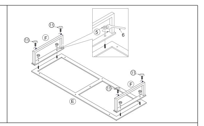
Assemble the Bottom Metal Plate (E) and the iron leg (F) with a nut⑤ and tighten it with ahex wrench⑥, then rotate foot pad ① into foot (F).
