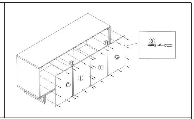
Fasten the Left and right side backboards (G) and Backboard Buckle (H) with csk screws®in turn.
