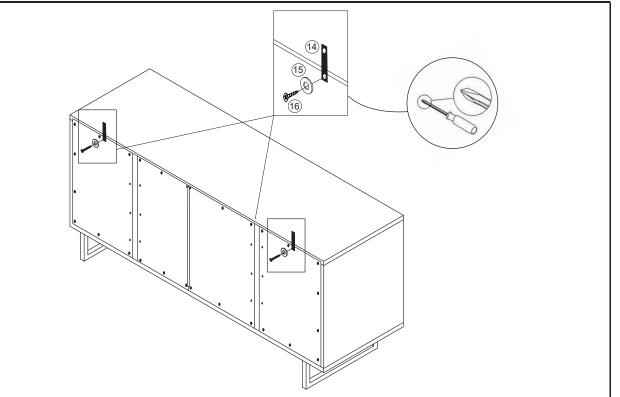
In the upper left and upper right corners of the back of the cabinet, secure the Anti-Tipping Cloth Strip 14 to the sideboard using screwdrivers 19, Screw 16 and Gasket 15.
