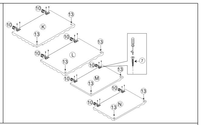
Fasten the door hinge ① with csk screws⑦ and the side holes of the door panel (K)(L) (M)(N).Attach Clear plastic gasket ① to the front and rear ends of the panel.
