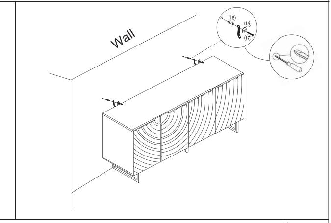
Align the cabinet with the wall and the strip. Screw the expansion screw 18 into the wall and install the flat gasket 15 and screw 17 using the Anti-reverse cloth strip 12 connected to the cabinet. Screw in the tilting strip with a screwdriver 19.
