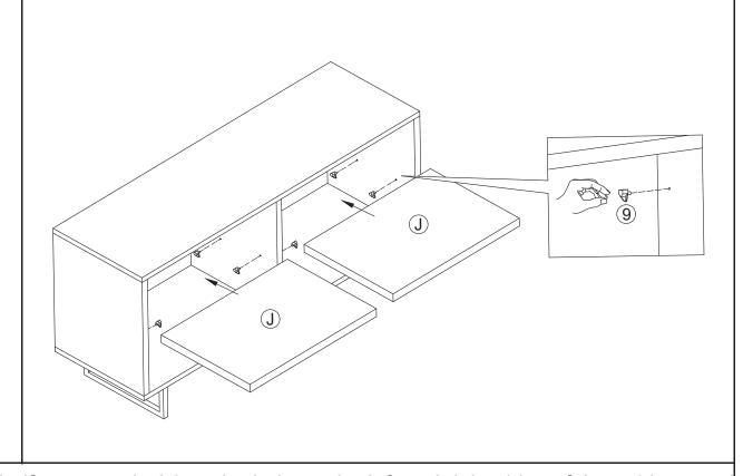
Insert the shelf support pin 9 into the hole on the left and right sides of the cabinet, and then place the shelf board (J) in.
