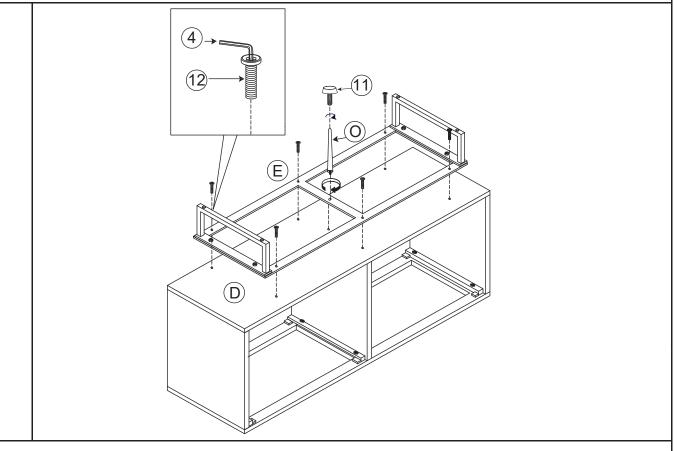
Align the installed Bottom Metal Plate (E) with the hole in the bottom board (D) and use screws (2) to tighten with Allen wrench (4). Finally, Rotate the middle leg (O) into the center hole, Rotate Foot Pad (1) into the Middle Leg (O) Position.
