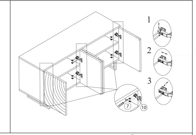
As shown in the picture, use Cak Screw 7 and a screwdriver 19 to connect the Door hinge 10 to the cabinet body with the door panel. Repeat the same steps to install all four door panels.
