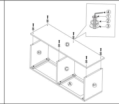
Place the bottom board (D) on the left and right side plates (B1)&(B2) and the middle board (C) to align the holes with screws1spring Leaf2flat gasket3to align the holes and tighten the fixed positions with a hex wrench4.
