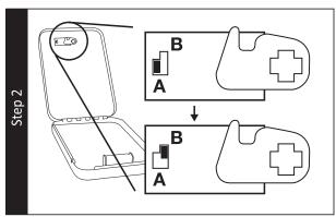
3. Set the combination to your new 3 digit combination. Once entered, while your vault is still open, turn the knob counterclockwise to lock. Finally, return the lever on the inside of the lock face from "B" to "A". Your new combination is now set.
