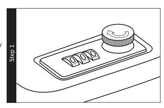
On the inside of the lock face, move the lever from the "A" to the "B" position. Your case is now ready to be progammed with a new, personal code.
