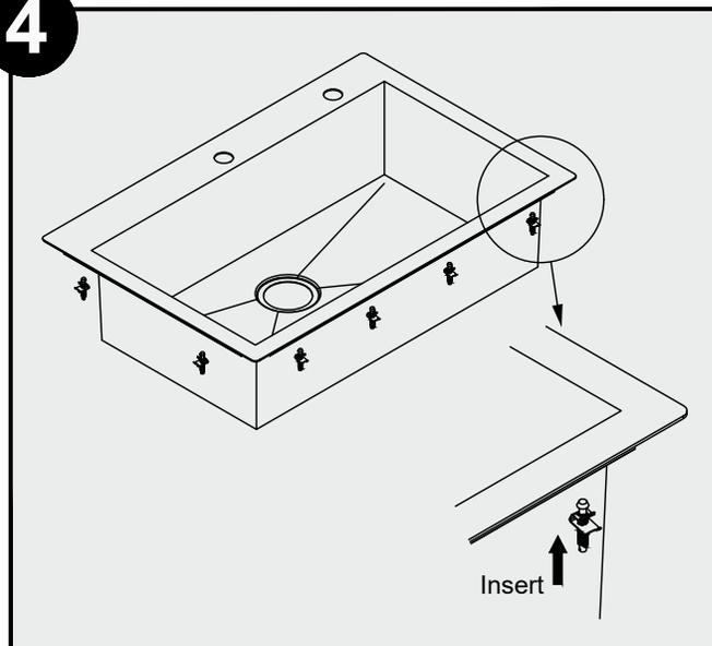
Attach the mounting hardware to the rails protruding from the underside of the sink rim. Make sure the hooked side of the mounting clip is facing away from the sink.
