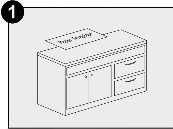
Locate the cutout template in the box and check with sink for accuracy. Cut carefully along the dotted lines. Place the template on the counter, in the location where you will be installing the sink. When placing the template, note the location of cabinet doors and panels to ensure that they are compatible with sink installation. Fix the template to the counter using masking tape.
