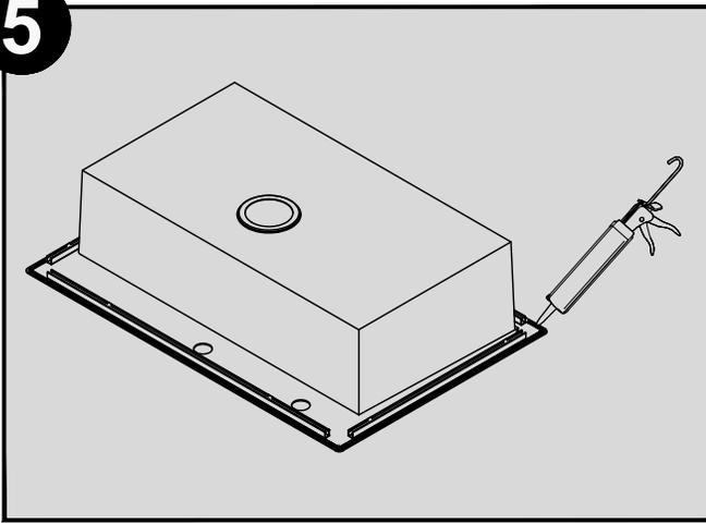
Clean and dry the surface around the opening of the sink. Verify that the sink fits correctly in the opening. The edge of the sink must sit on the counter. Turn the sink upside down to apply sealant. Apply silicone-based sealant (not included) underneath the edge of the sink rim.
