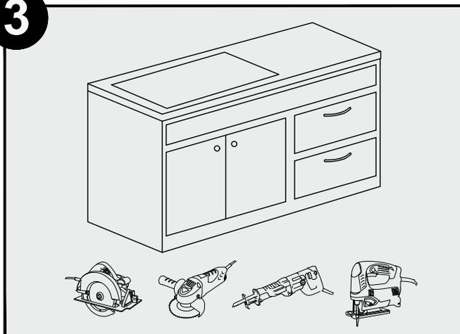
Cut the opening in the countertop by carefully following the traced line. Cut the countertop using the appropriate cutting tools.
