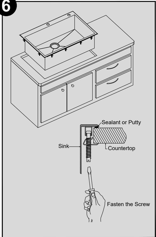
Insert the sink into the opening, check the alignment of the sink to the cutout in the countertop and press firmly. Tighten the screws in the front of the sink, followed by the ones in the back and on the sides of the sink. Remove any excess silicone-based sealant. Allow the sealant to set for 30-60 minutes.
