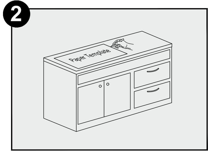
Trace the template with a marker pen. Remove the template from the countertop. If using a CNC machine, download the DXF file from [www.karran.com](http://www.karran.com) and proceed accordingly.
