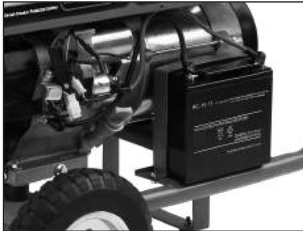
Put the battery on the frame, have the battery assembled with the provided accessories as shown.
