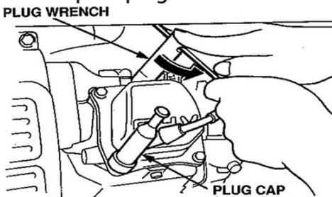
4. Visually inspect the spark plug. Discard it if the insulator is cracked or chipped. Clean the spark plug with a wire brush if it is to be reused.
