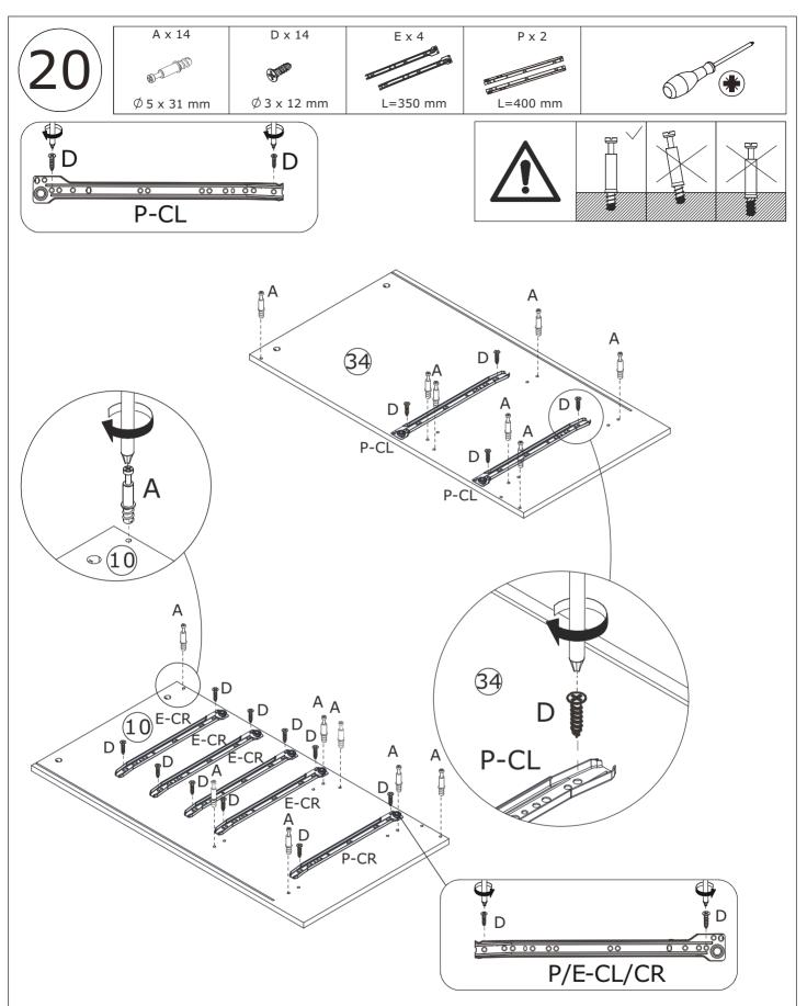
Fix slide rail(P-CL) to plate 34 using screw(D) as shown. Fix slide rail(E-CR) and (P-CR) to plate 10 using screw(D) as shown.
