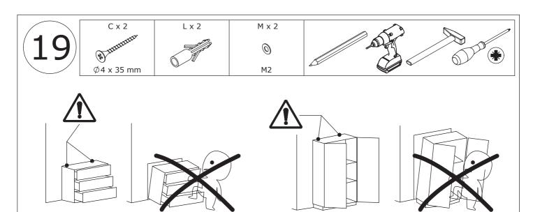
Once assembled lift furniture into place, do not drag. Use a drill to create a small hole lining up with the top of the safety strap (M3). Fasten to wall using wall anchor (L), washer (M2), wall screw(C). Ensure the unit is balaced and steady before use. You're done, enjoy
