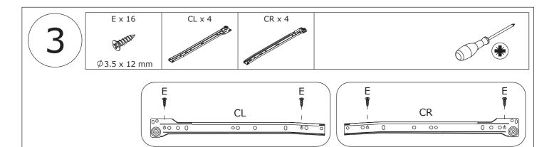
Fix rail(CL) to board 12(board 2) and 5 with screw(E) as shown. Fix rail(CR) to board 12(board 3) and 4 with screw(E) as shown.
