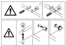
Cover board 1 to top using wooden dowel(D), add cam lock(B) into board 6 and turn clockwise to tighten as shown.
