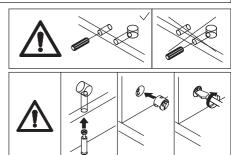
Attach board 6 to board 5 using wooden dowel(D), add cam lock(B) into board 6 and turn clockwise to tighten as shown.
