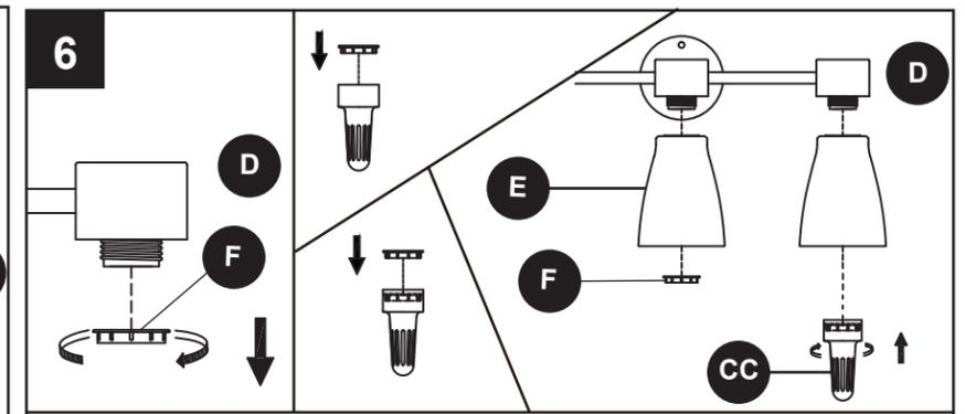
**!** Unscrew the socket rings (F) from sockets on fixture body (D). Attach glass shades (E) over the sockets. Tighten socket rings (F) with socket ring fastener (CC) as needed.
