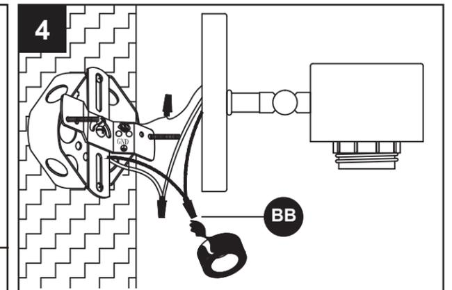
**!** Attach (BB) to connections with electrical tape (not included).
