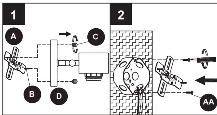
**!** Attach (A) to outlet box using (AA). Temporarily place (D) through (B).
