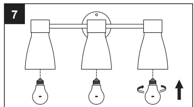
**!** Install light bulbs (not included). Use 60-watt max. standard-base incandescent bulbs or CFL/LED equivalents.
