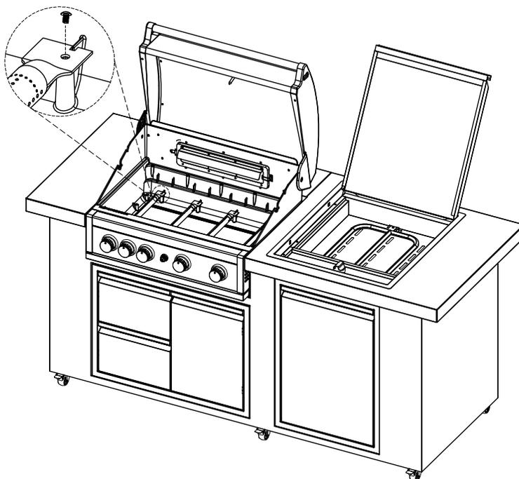
Step 3: Remove the burners.
