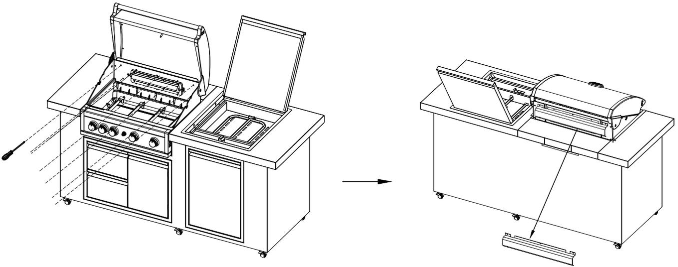
Step 2: Use the 7mm wrench provided to remove the propane orifice.
