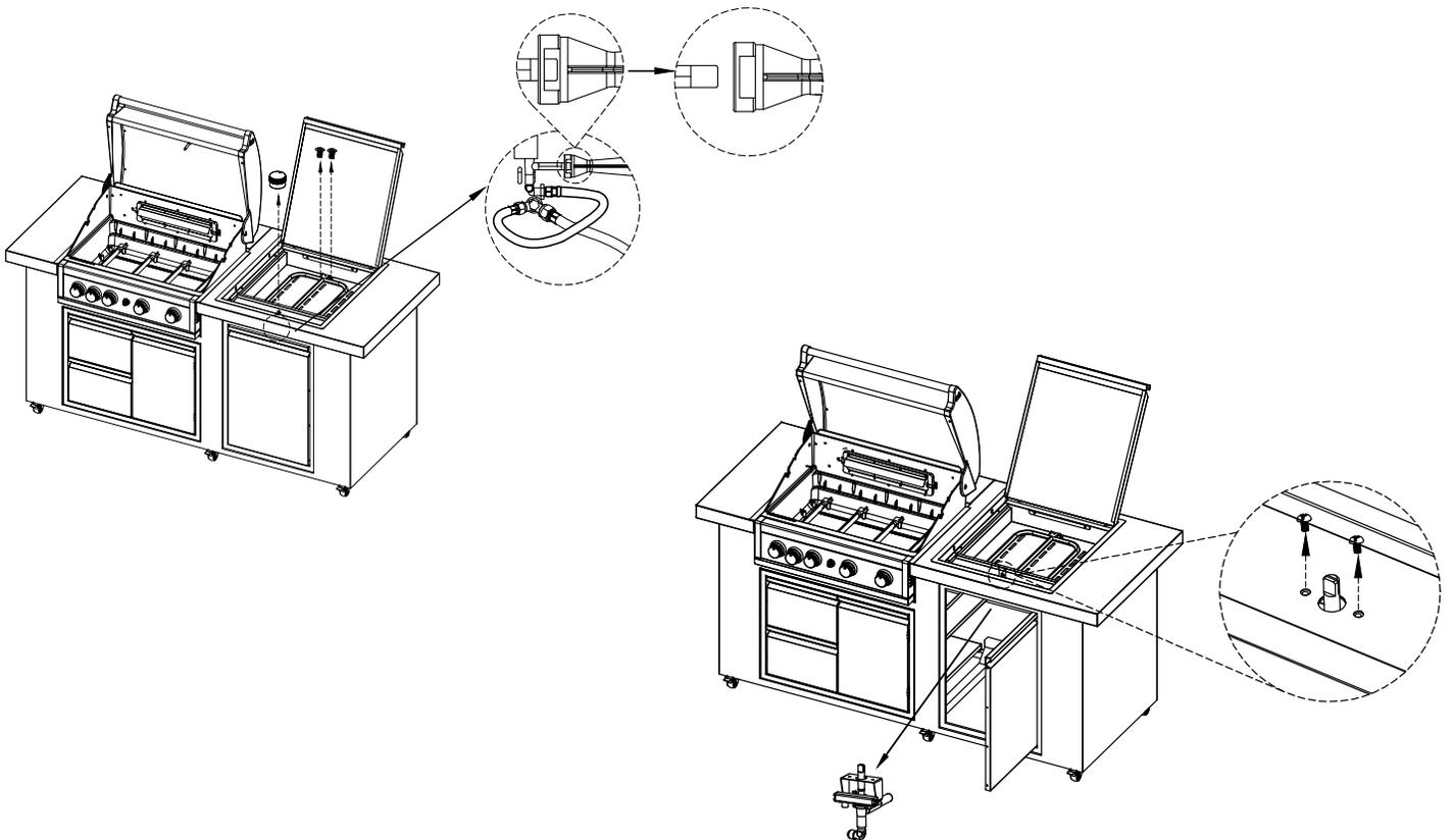
**Replace with Natural gas griddle burner valve**
