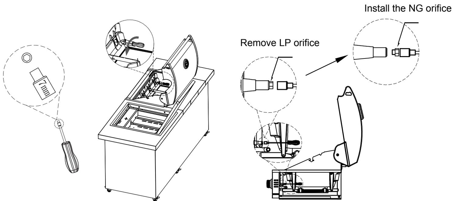
Step 5: Remove the control knobs and use flathead tool to make two counterclockwise turns. Turning this will allow natural gas to flow when it is connected.
