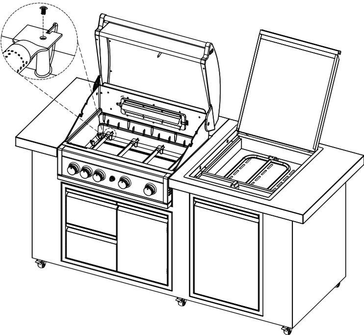
Step 8: Install the control knobs.
