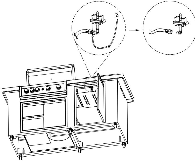
Step 12: Remove 2 screws to remove the **griddle burner**.
