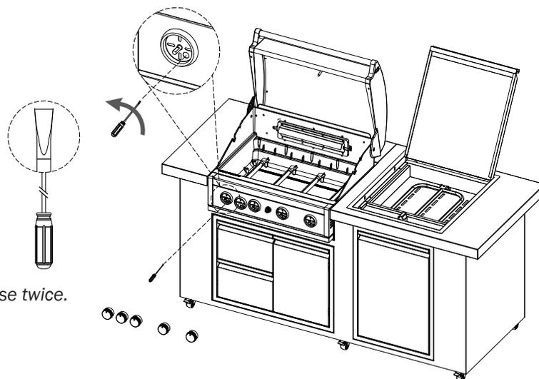
Step 6: Install the burners.
