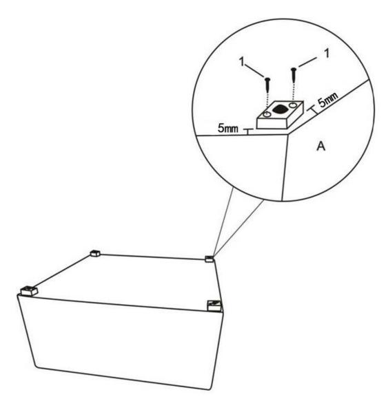
Place the Ottoman (A) on its back on a flat smooth surface. Attach Ottoman Feet (C) to Ottoman (A) with Self-tapping Screw (1) to each corner using a Screwdriver.
