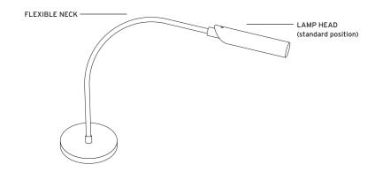
To set the light at different positions - bend any part of the "FLEXIBLE NECK" to move it. Never apply force to the "LAMP HEAD" to redirect the light. The "LAMP HEAD" can be gently adjusted downward from the "standard position" by 90 degrees and side-to-side by 270 degrees.
