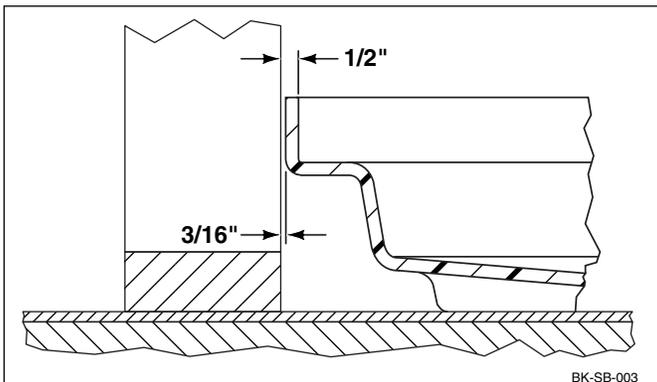
2. After the shower floor installation is complete, install 1/2" moisture-resistant wall board, as shown. The ideal installation results when the outside surface of the wall board and shower floor flange are flush, as shown in the illustration below.
