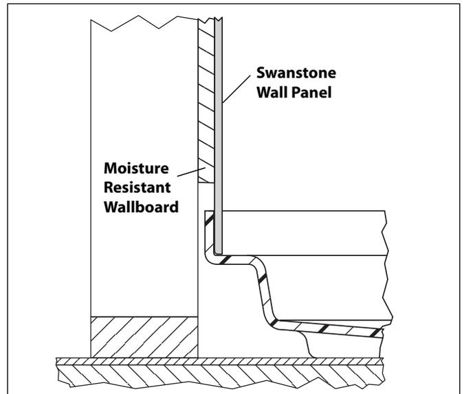
**Note:** The barrier-free shower floor ramp can be installed on the same floor surface as the shower floor or can be installed on raised floor surface (up to 1/2" thick), as shown below.
