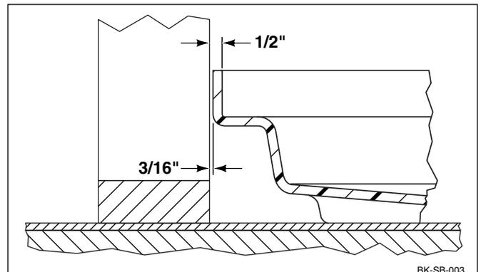
**Note:** When constructing or modifying stud wall framework, make sure to install (gang) multiple studs to provide support for any required moisture resistant wall board, solid surface panel attachment flanges, or filler boards, etc. Framework depth (B) must be at least 3/16" more than the actual depth measurement of the shower floor.
