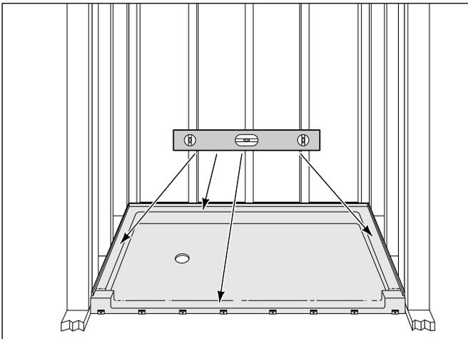
**Note:** Clean up any excess mortar/thinset and allow the mortar/thinset under the barrier-free shower floor ramp to cure for 24 hours.
