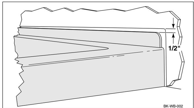
3. The Swanstone or alternate shower wall material will be installed over the 1/2" moisture-resistant wall board and shower floor flange, as shown in the illustration below.
