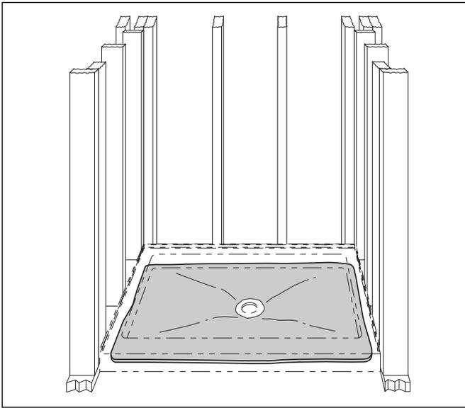
3. Place the shower floor into the rough opening and firmly press it into the mortar/thinset. The exposed front bottom edge(s) of the shower floor should contact the subfloor.
