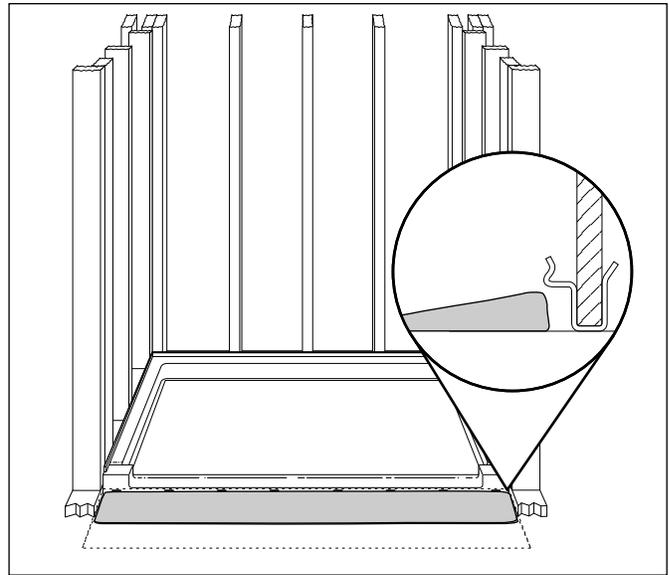
6. Apply a bead of 100% silicone sealant to seal the joint between the shower floor and shower floor ramp.
