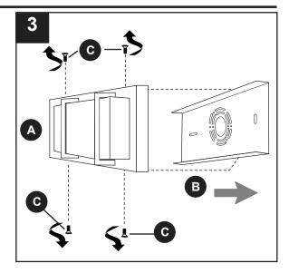
Attach mounting plate (B) to outlet box (not included) using existing washers and outlet box screws or the machine screws (BB).
