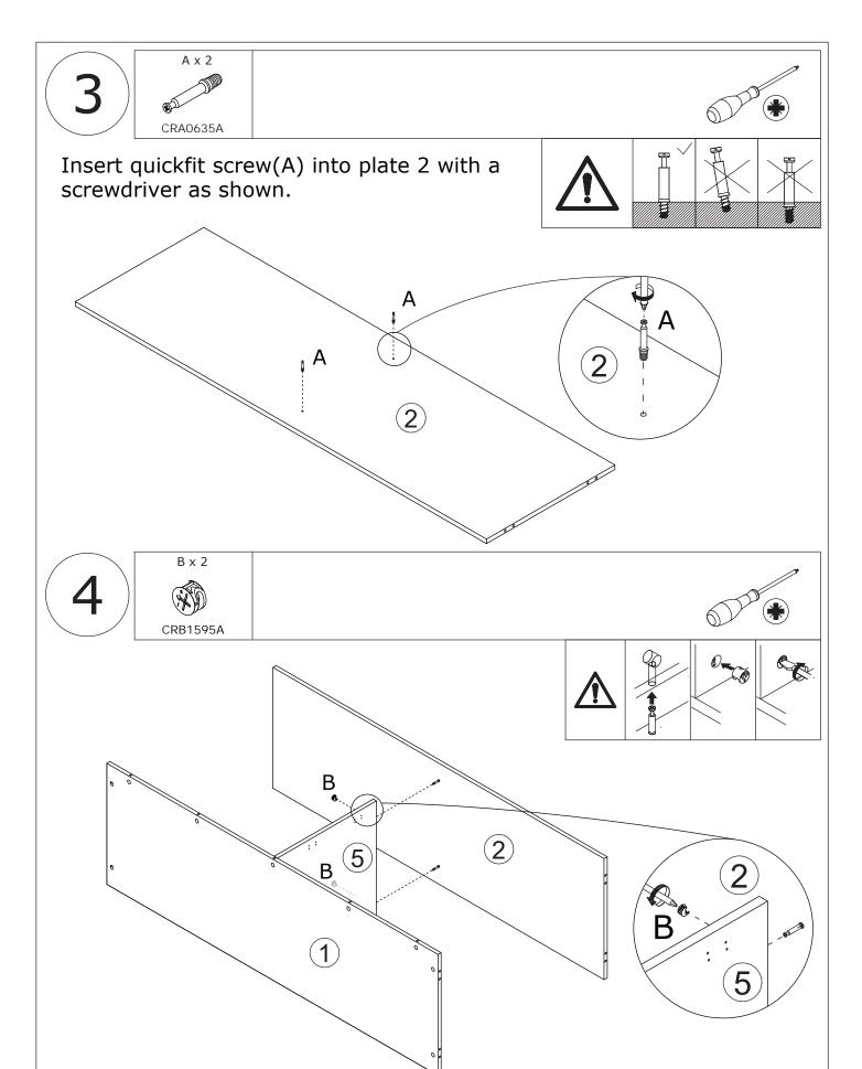
Attach plate 2 to plate 5, put cam lock(B) into holes in plate 5 and turn clockwise to tighten as shown.
