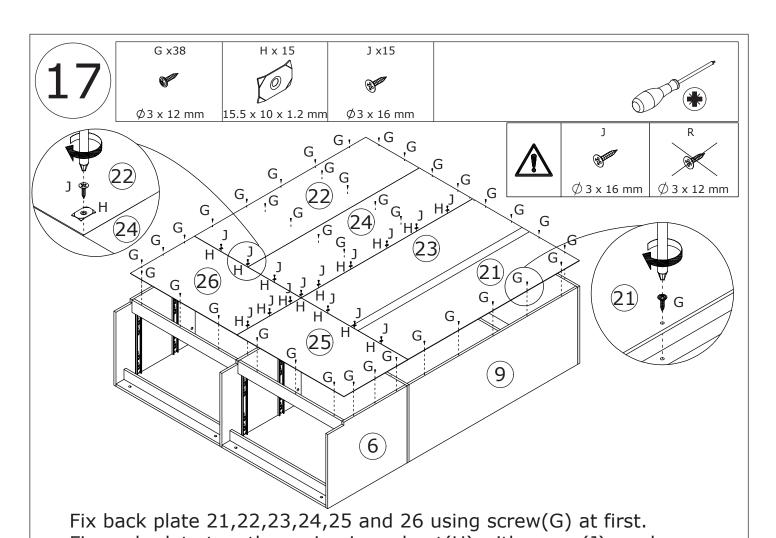
Fix each plate together using iron sheet(H) with screw(J) as shown.
