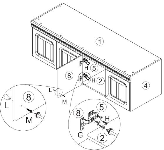
Attach another plate 8 to plate 5 by fixing hinge(G) with screw(H) as shown.Fix knob(L) to door plate with screw(M) as shown.
