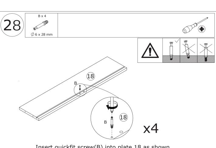
Insert quickfit screw(B) into plate 18 as shown.
