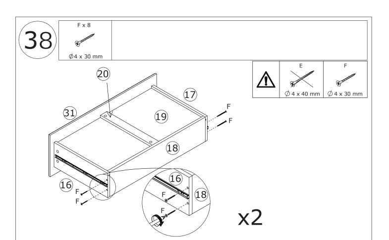
Fix plate 18 to plate 16 and 17 with screw(F) as shown.
