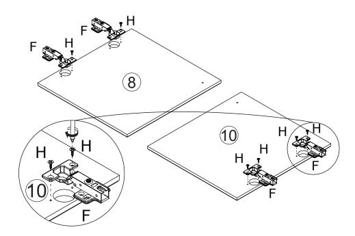
Fix hinge(F) to plate 8 and 10 respectively with screw(H) as shown. Please note, hinge(F) is used in this step.
