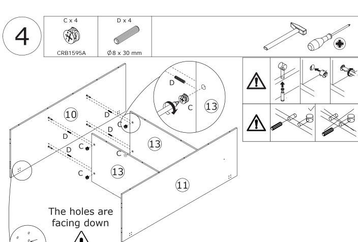
Attach plate 10 to plate 13 with wooden dowel(D) at first.
