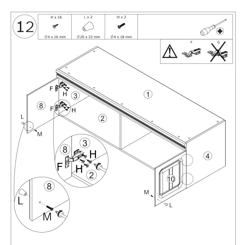
Attach plate 8 to plate 3; plate 10 to plate 4 by fixing hinge(F) with screw(H) as shown.
