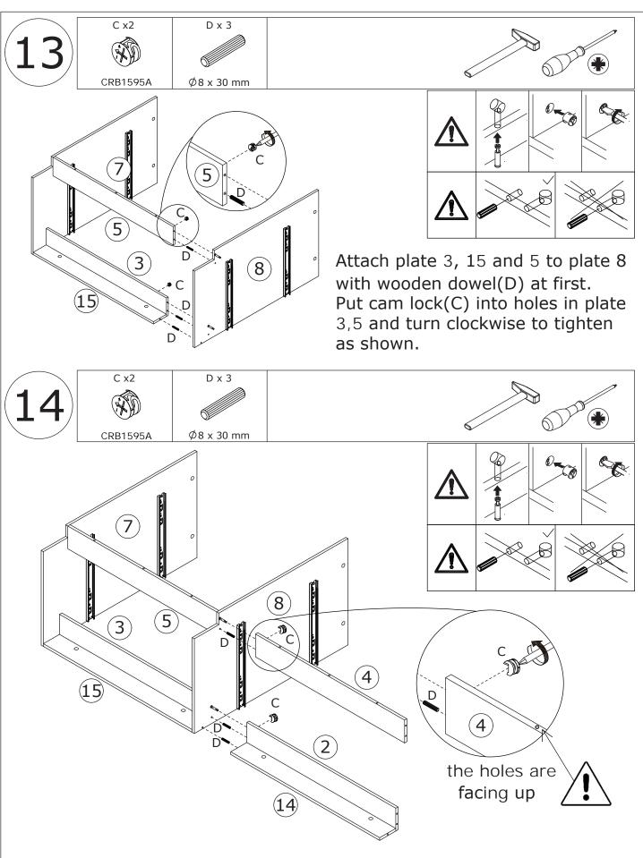
Attach plate 2, 14 and 4 to plate 8 with wooden dowel(D) at first. Put cam lock(C) into holes in plate 2,4 and turn clockwise to tighten as shown.
