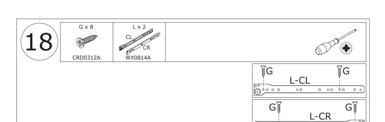
Fix rail(CL/CR) to panel 3, 4 and 5 with screw(G) as shown.
