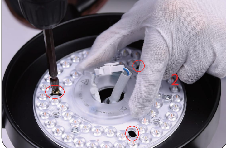
12. Insert three light kit screws, and then tighten them
